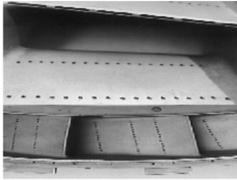
Fig. 2.1: Showing small angular holes of a turbine component
