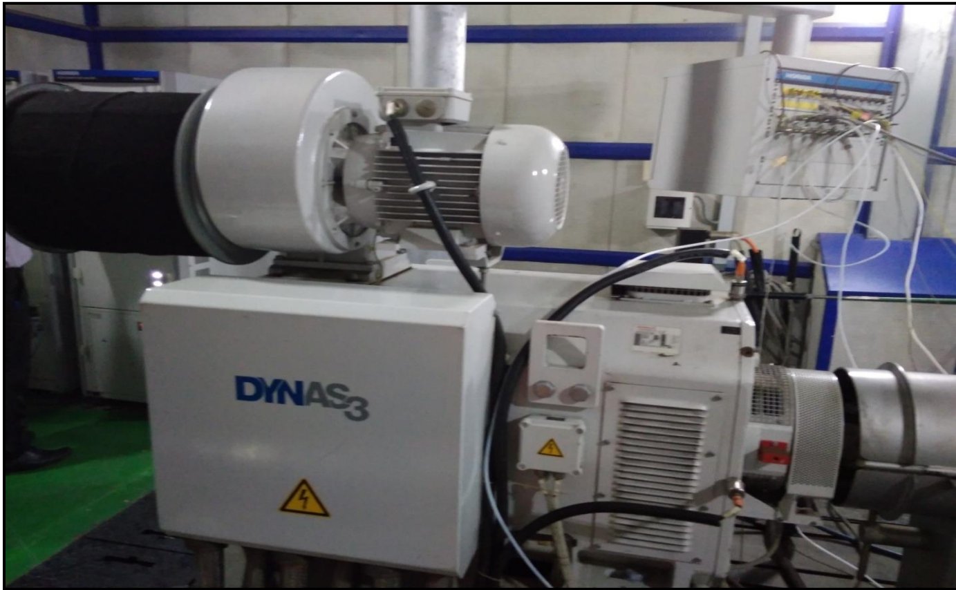
Figure 4.2 Transient AC asynchronous dynamometer
