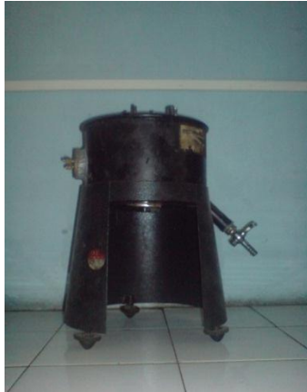
Plate 3.1: Redwood Viscometer Used for Measurement of Kinematic Viscosity
