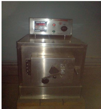
Plate 3.6: Muffle Furnace Used for Measurement of Ash Content
