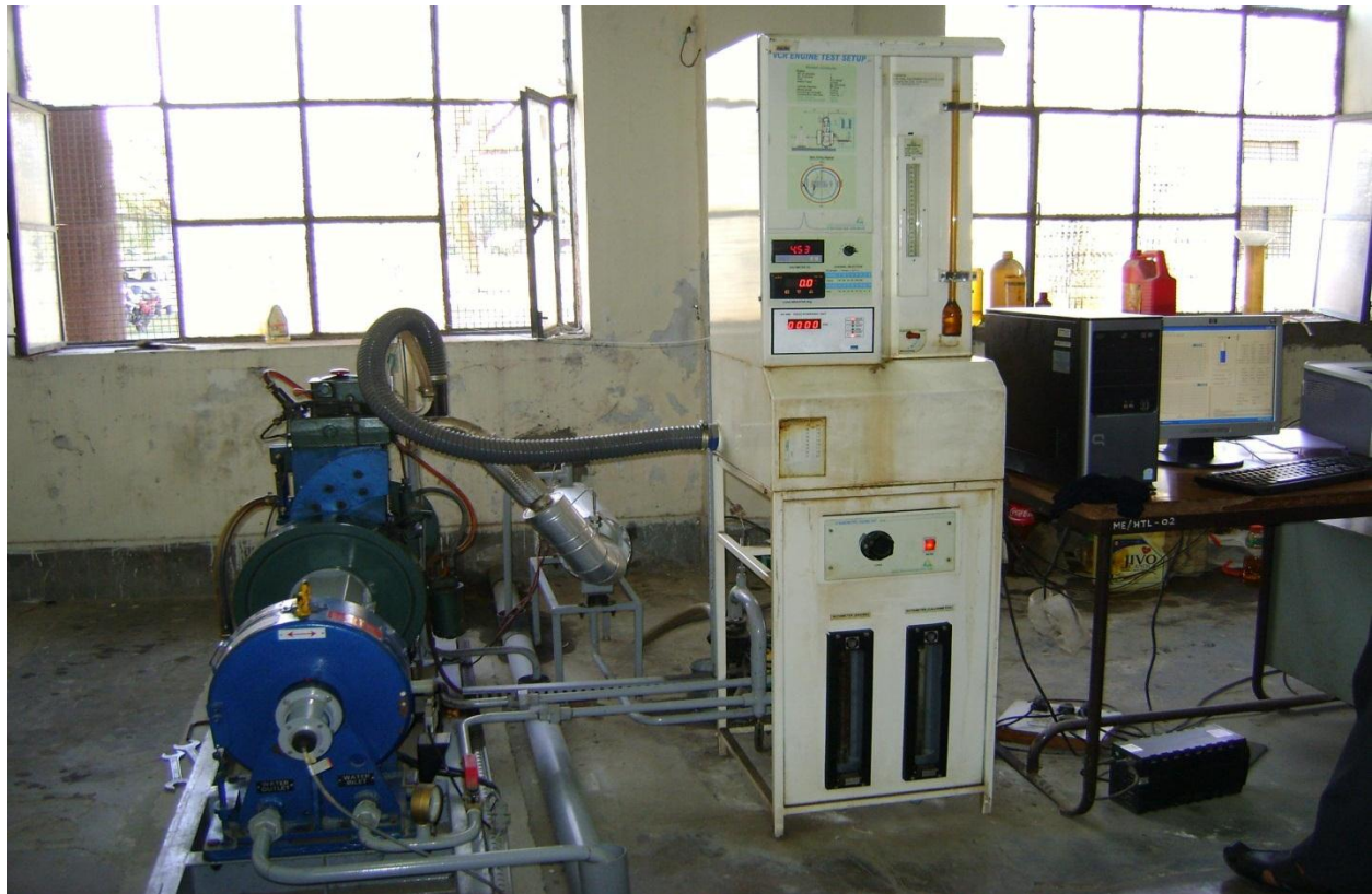
Plate 3.7: Variable compression ratio compression ignition engine experimental setup
