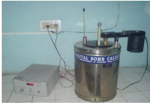
Plate 3.2: Digital Bomb Calorimeter Used for Measurement of Calorific Value
