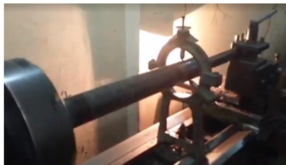
Figure 2.17 : Boring of 3-inch pipe
