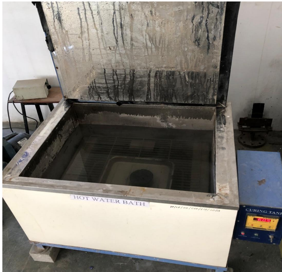
Figure 4.7 : Specimens at 60^{\circ}\text{C} water bath
