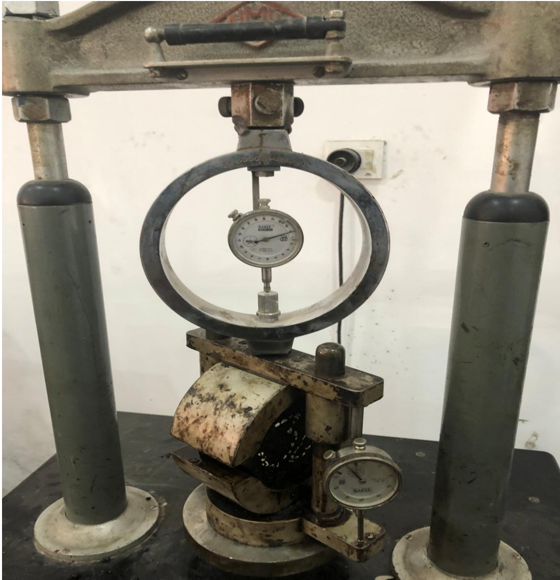
Figure 4.8 : Marshall testing for specimens
