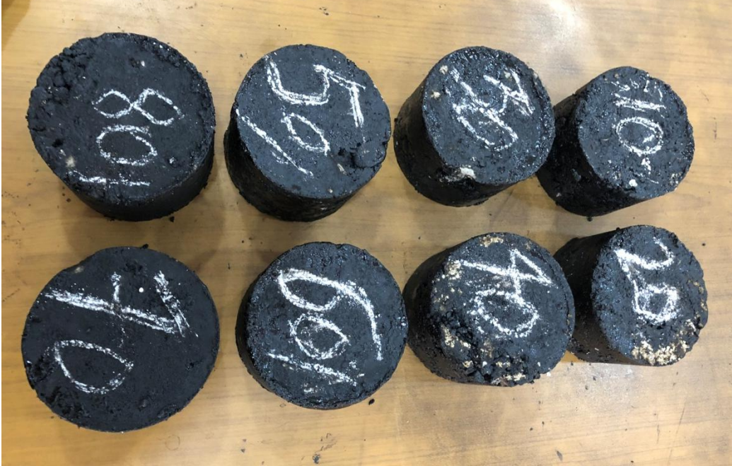
Figure 4.4 : Modified compacted mixes with Saw Dust Ash and Hydrated Lime filler
