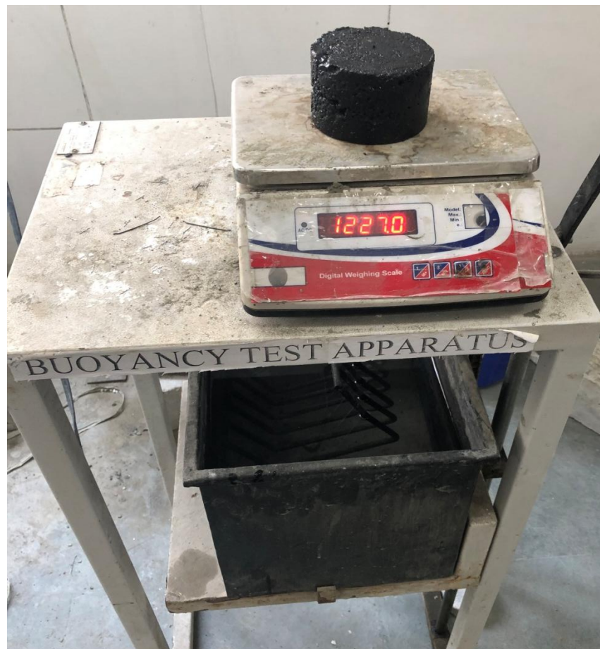
Figure 4.6 : Saturated surface dry weight for Bulk specific gravity
