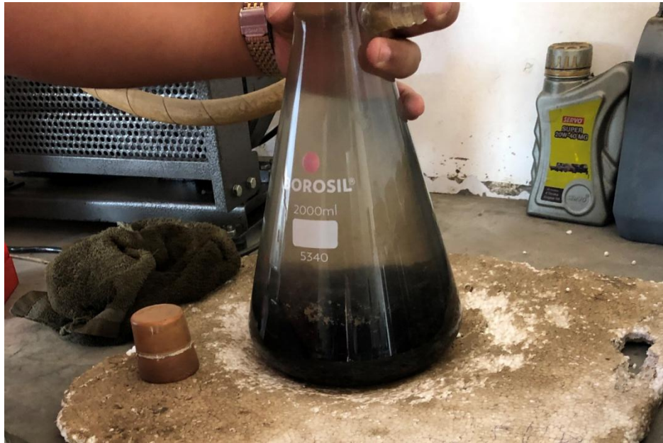
Figure 4.9 : Theoretical Maximum Specific Gravity test for specimen
