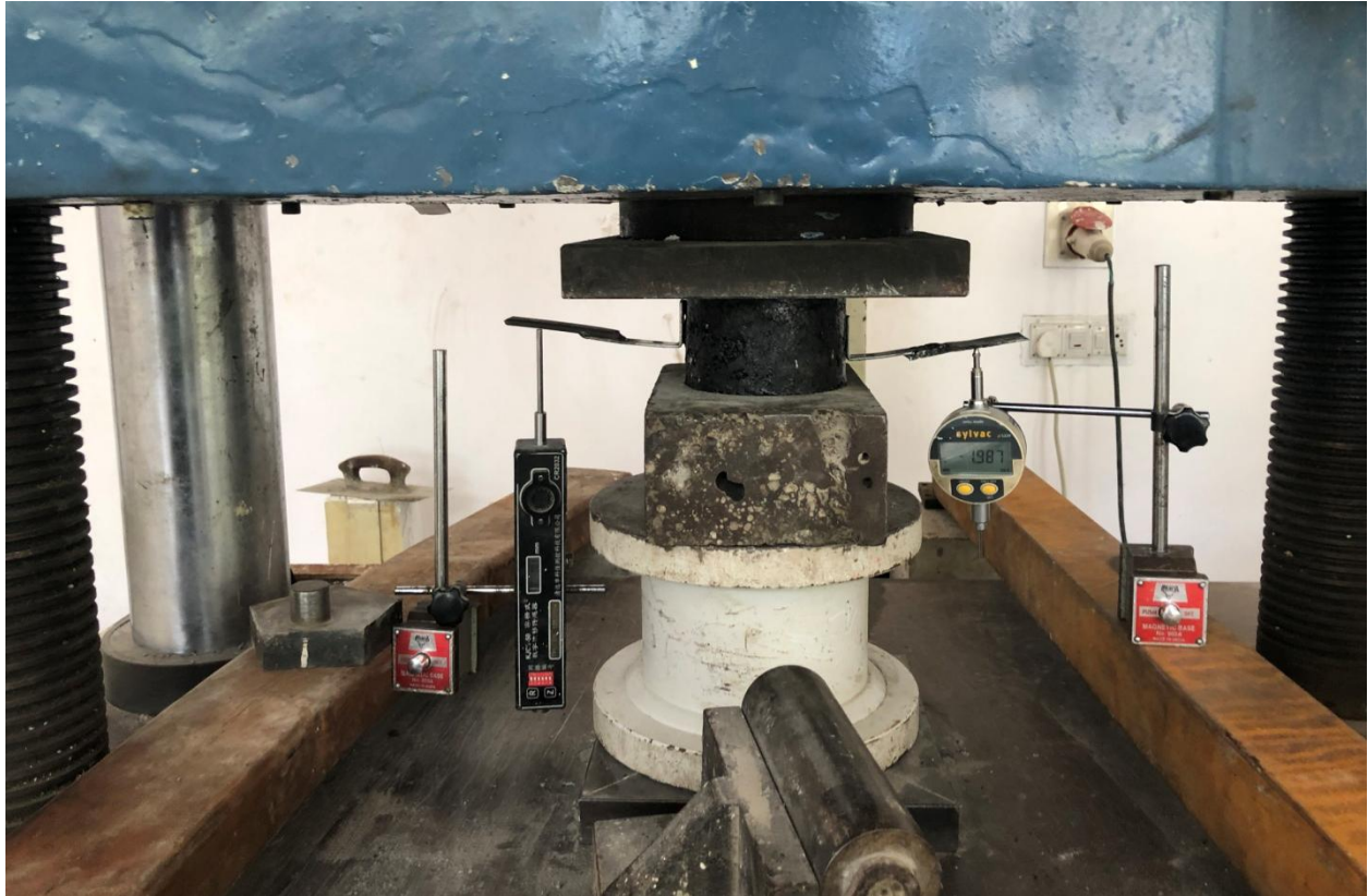
Figure 4.10 : Specimen setting under UTM
