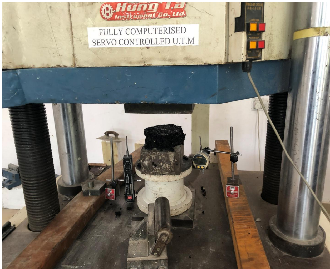
Figure 4.11 : Failed specimen under UTM test
