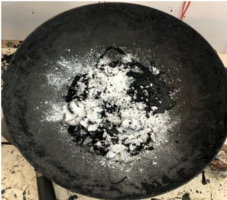
Figure 4.2 : Modified mix while heating with Saw Dust Ash and Hydrated Lime
