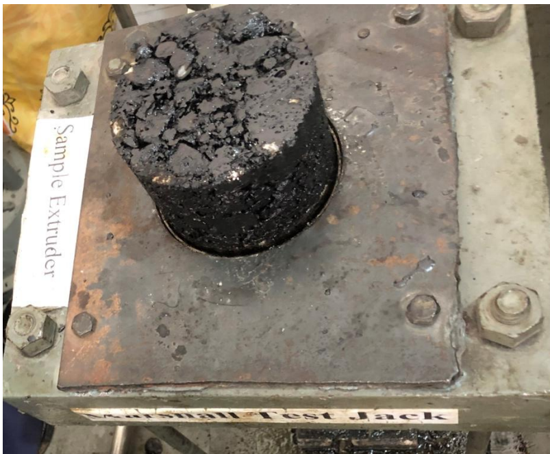
Figure 4.5 : Sample extraction from extruder
