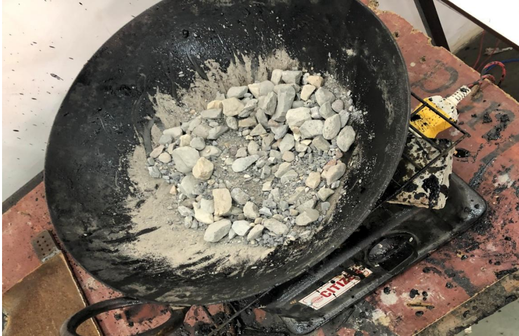
Figure 4.1 : Unmodified mix with Stone Dust
