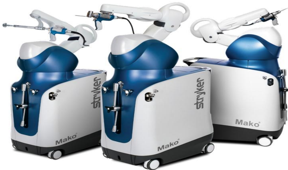
Figure 1. 1 MAKO Robot (Total Hip Arthroplasty and Total Knee Arthroplasty) [MAKO THA Surgical Guides]
