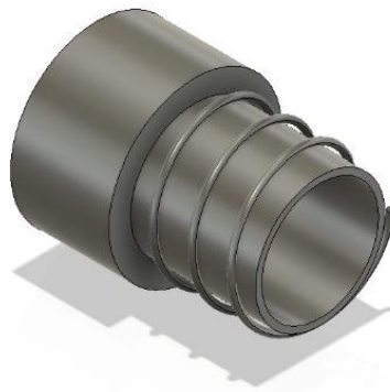
Figure 4. 6 - Spring placement within Hip Chuck Slide Assembly
