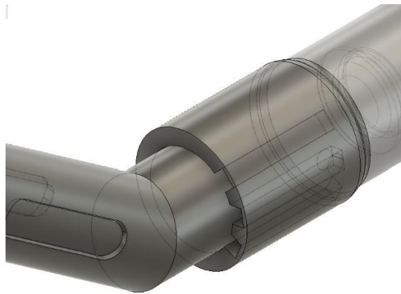
Figure 4. 3 - Locking Mechanism with Internal Spline Engagement
