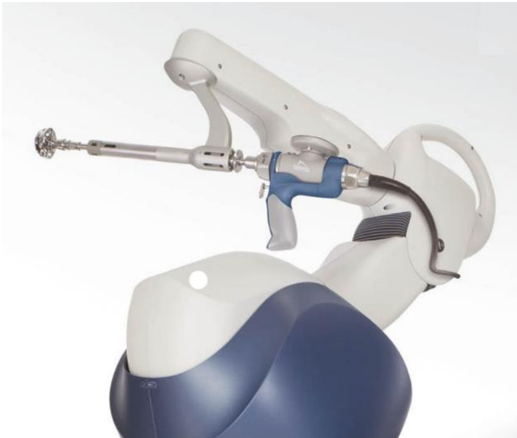
Figure 3. 2-Fully Assembled Reamer and Power Equipment in MAKO [18]
