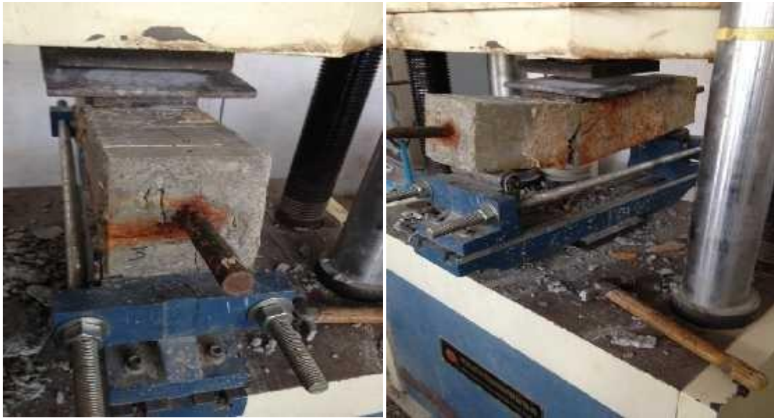
Fig.5.7 Beams under 2 point load testing
