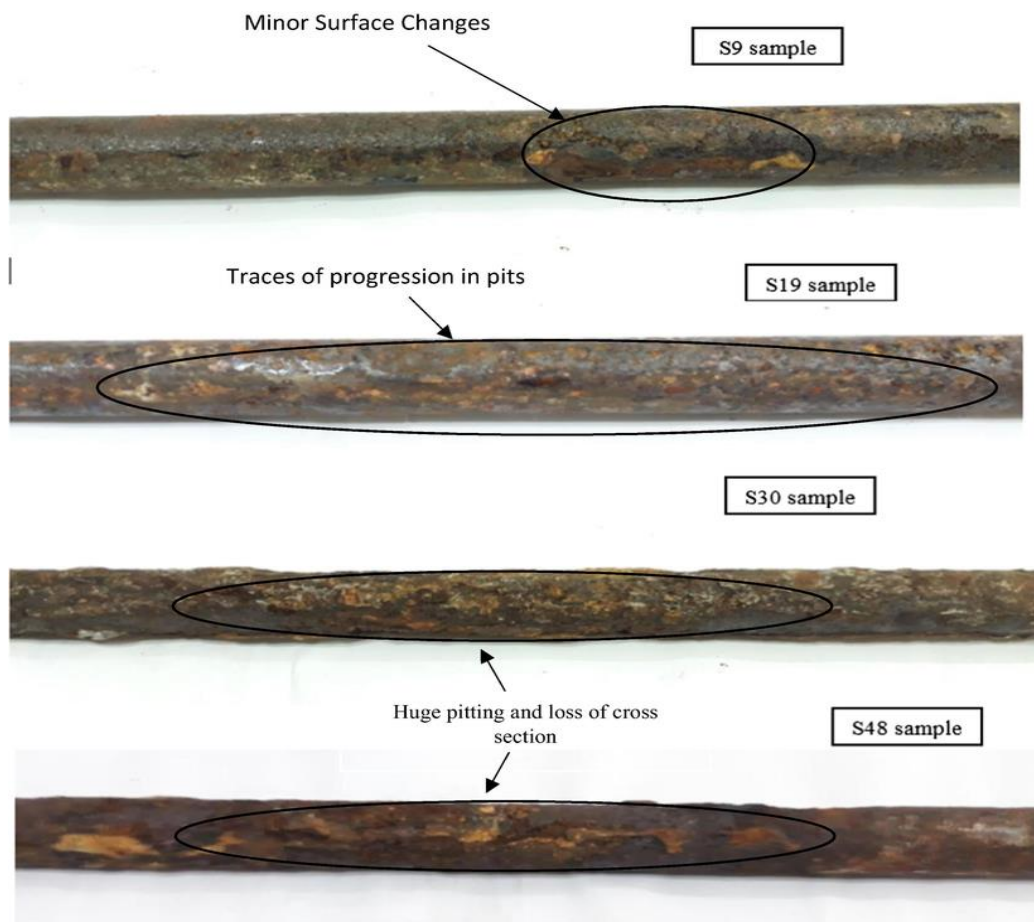
Fig. 4.11 Visual condition of the extracted bars at different ages of corrosion
