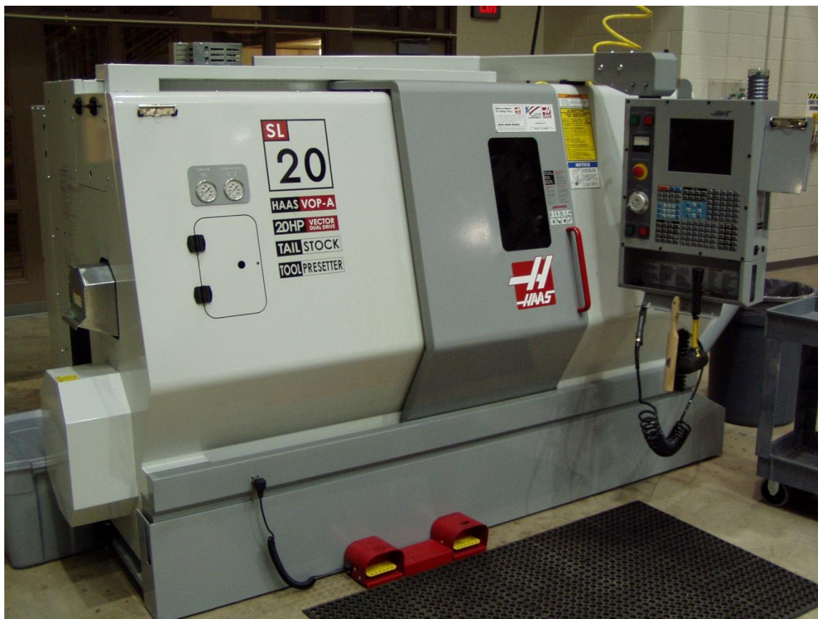
Figure 4: CNC TURNING CENTER [W5]
