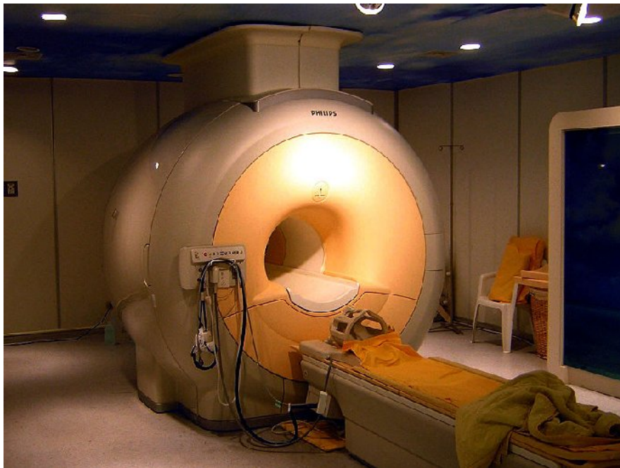
Figure 3.2: Modern 3 tesla clinical MRI scanner
