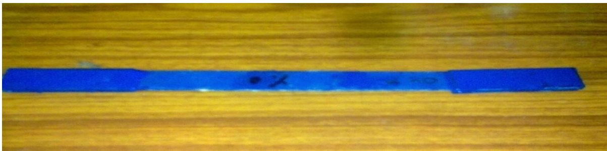
Fig.4.10: Nanocomposite specimen for tensile testing
