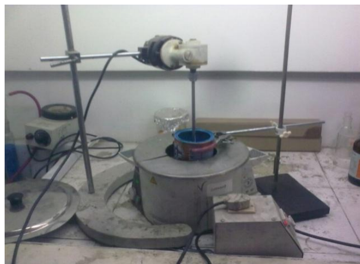
Fig. 4.1: Mechanical stirrer with oil bath set-up
