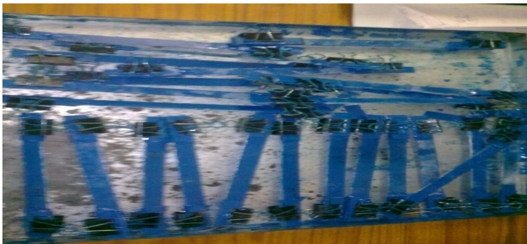
Fig. 4.11: Sample tabbed, Clamped and left for drying
