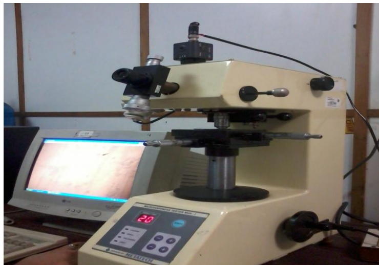
Fig. 4.16: Micro hardness tester
