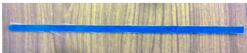
Fig.4.7: Nanocomposite flexural specimen
