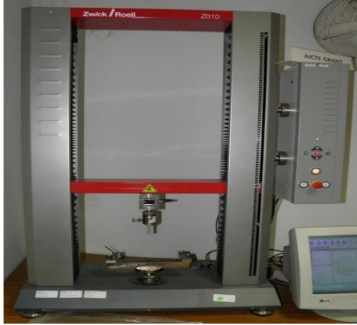
Fig. 4.14: UTM flexural setup
