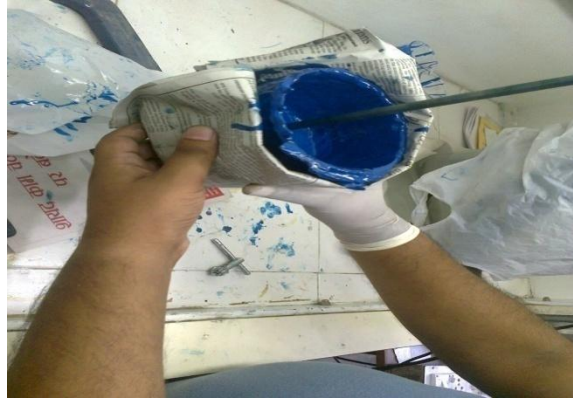
Fig. 4.3: Hardener mixing in Epoxy-Nanoclay base
