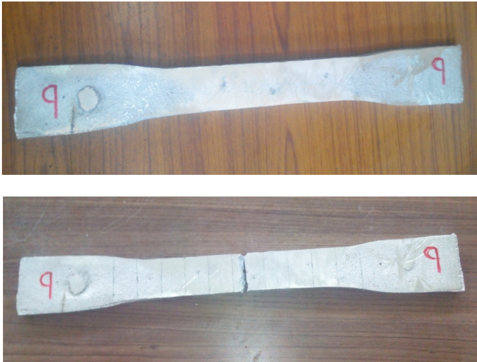
Figure 4.15: Tensile Test Specimen before and after the Test.
