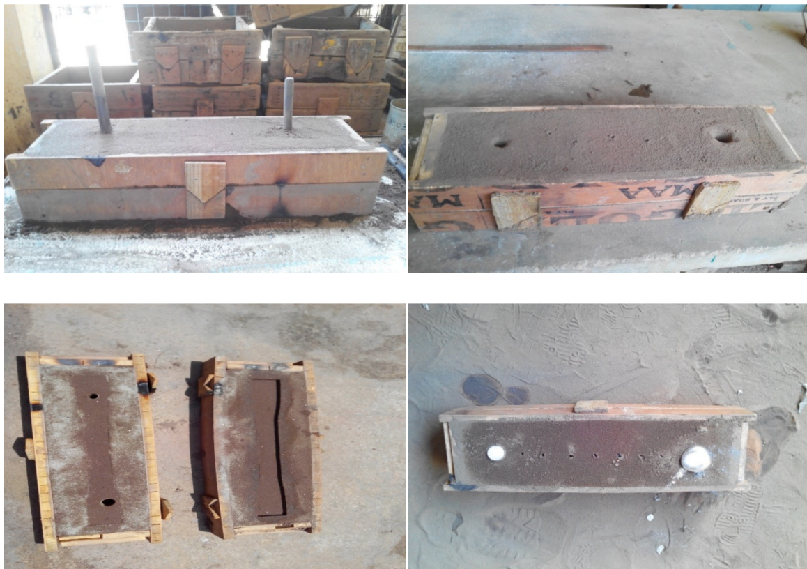
Figure 4.14: Mould Preparation and Casting of Samples
