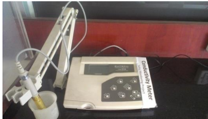
Figure 3.2 Electrical conductivity meter
