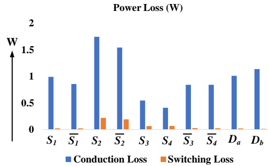
Fig. 5.7: Switching and conduction power loss of the proposed topology
