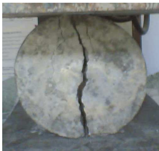
Fig. 4.6 Splitting Tensile Failure of cylinder
