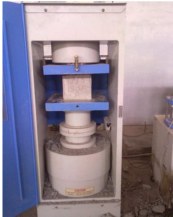
Fig. 4.2 Compressive strength test in progress
