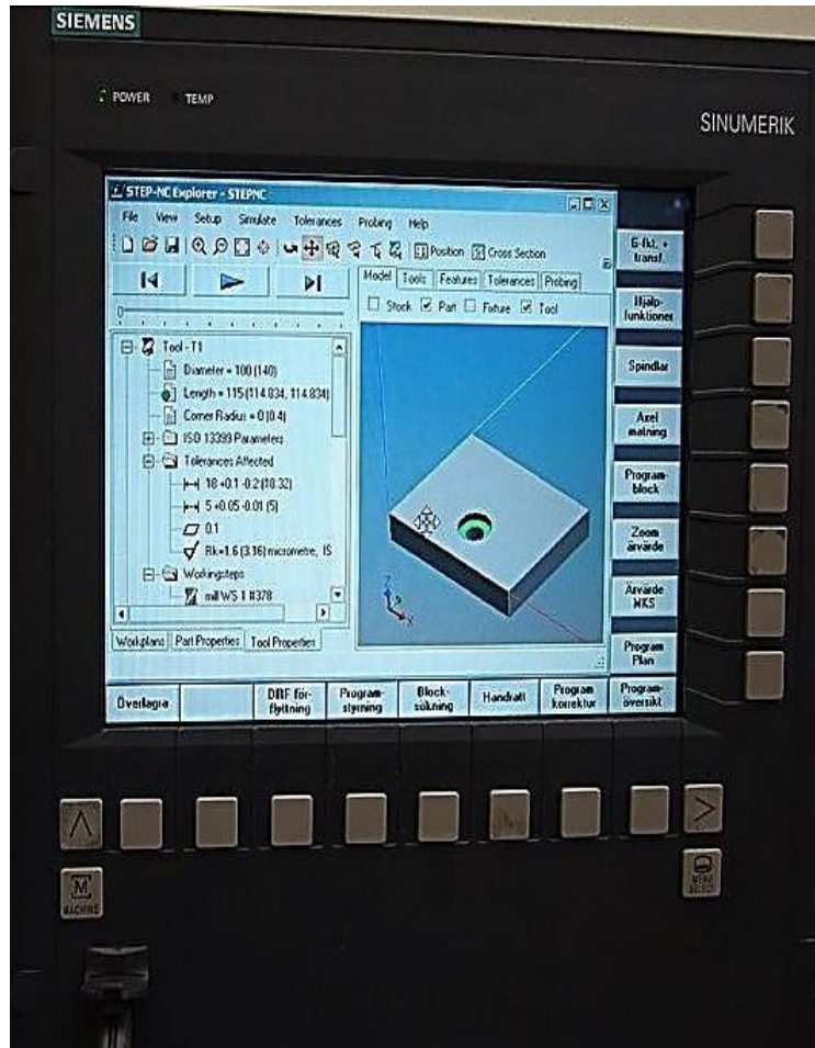
Figure 2.5: A Siemens Machine Having a Step NC Controller [w6]
