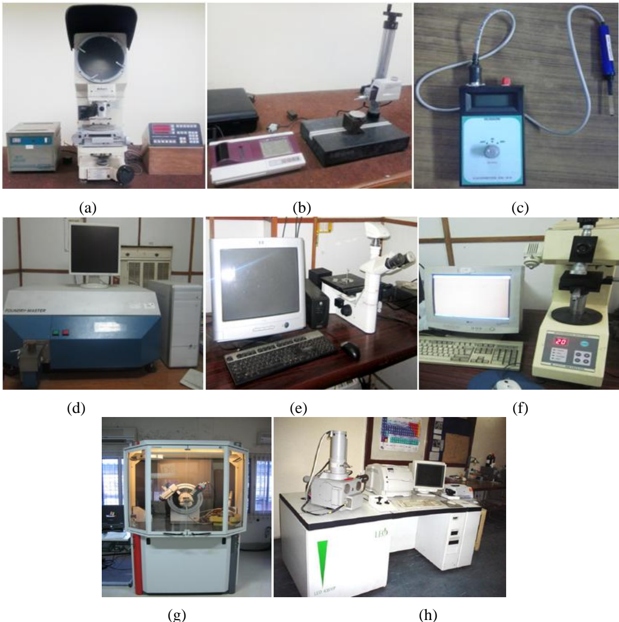
Figure 3.7: Measuring and test equipments (a) Profile projector; (b) Surface roughness tester; (c) Digital Gauss meter; (d) Optical emission spectroscope; (e) Metallurgical microscope; (f) Micro hardness tester; (g) X-Ray Diffraction machine; (h) Scanning Electron Microscope
