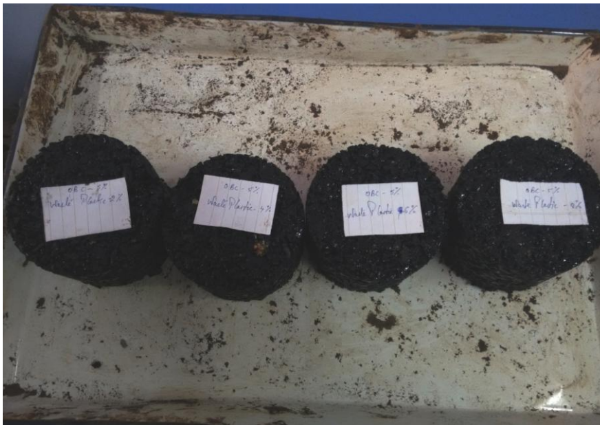
Plate 3.2 - Samples Extracted from Marshall Mould
