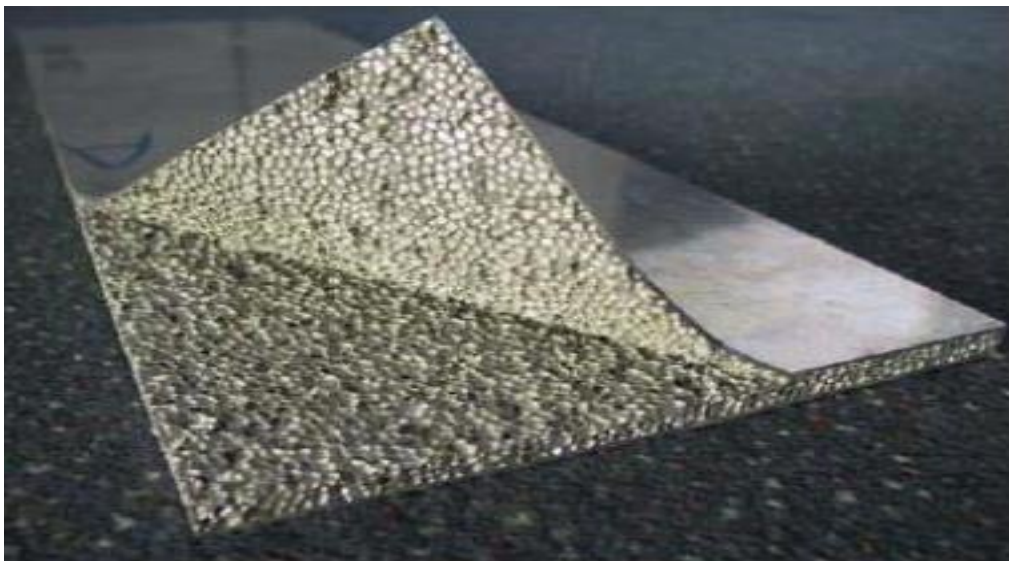
Figure 1.25: Ship's wall Al foam panel coatings for noise attenuation
