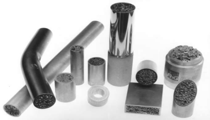
Figure 1.20: Several types of tubes and profiles - filled with aluminium foam. [Catriing Kammer, 1999]
