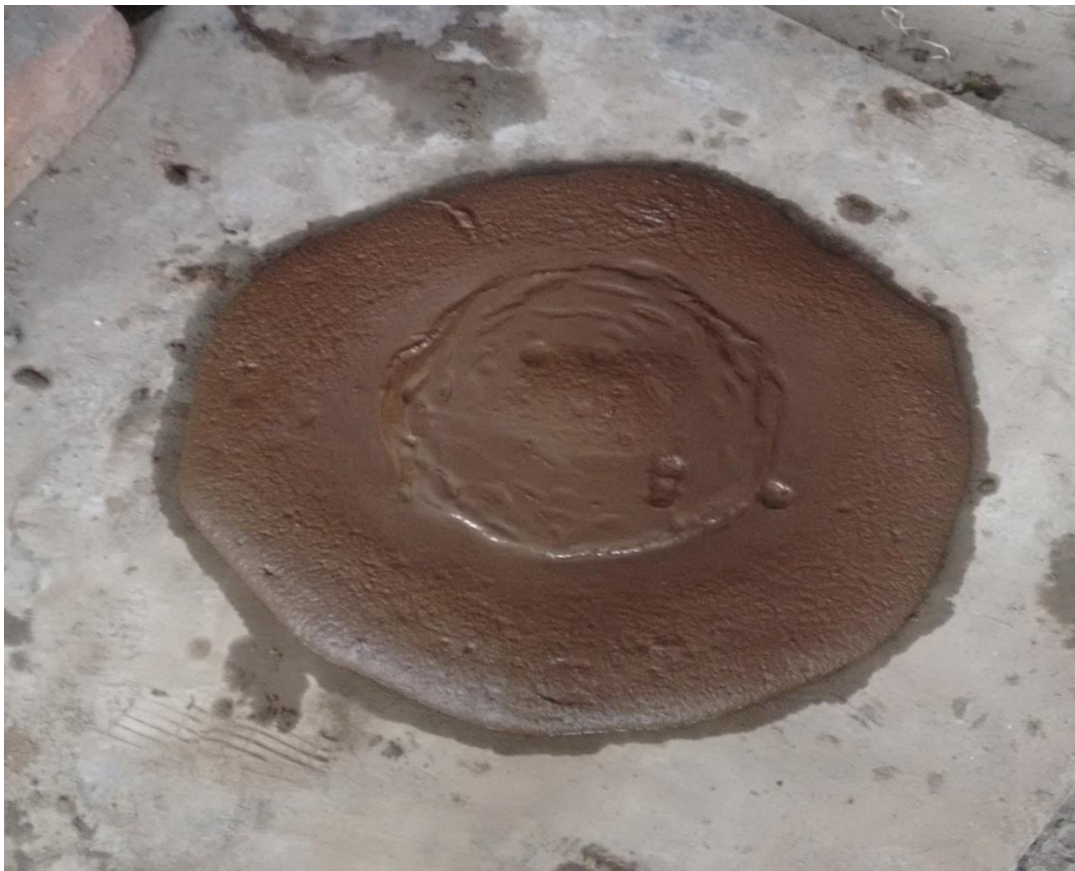
Figure 3.24: Flow table diameter observed for C/F/G 80A mix
