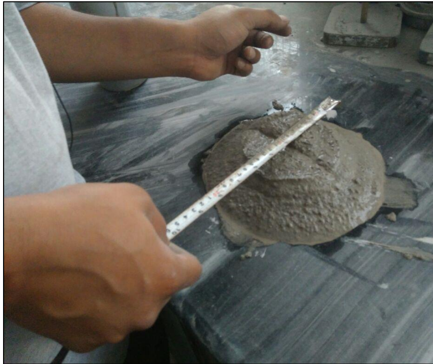
Figure 3.22: Cylinder slump flow test performed on C/R/G 100B mix
