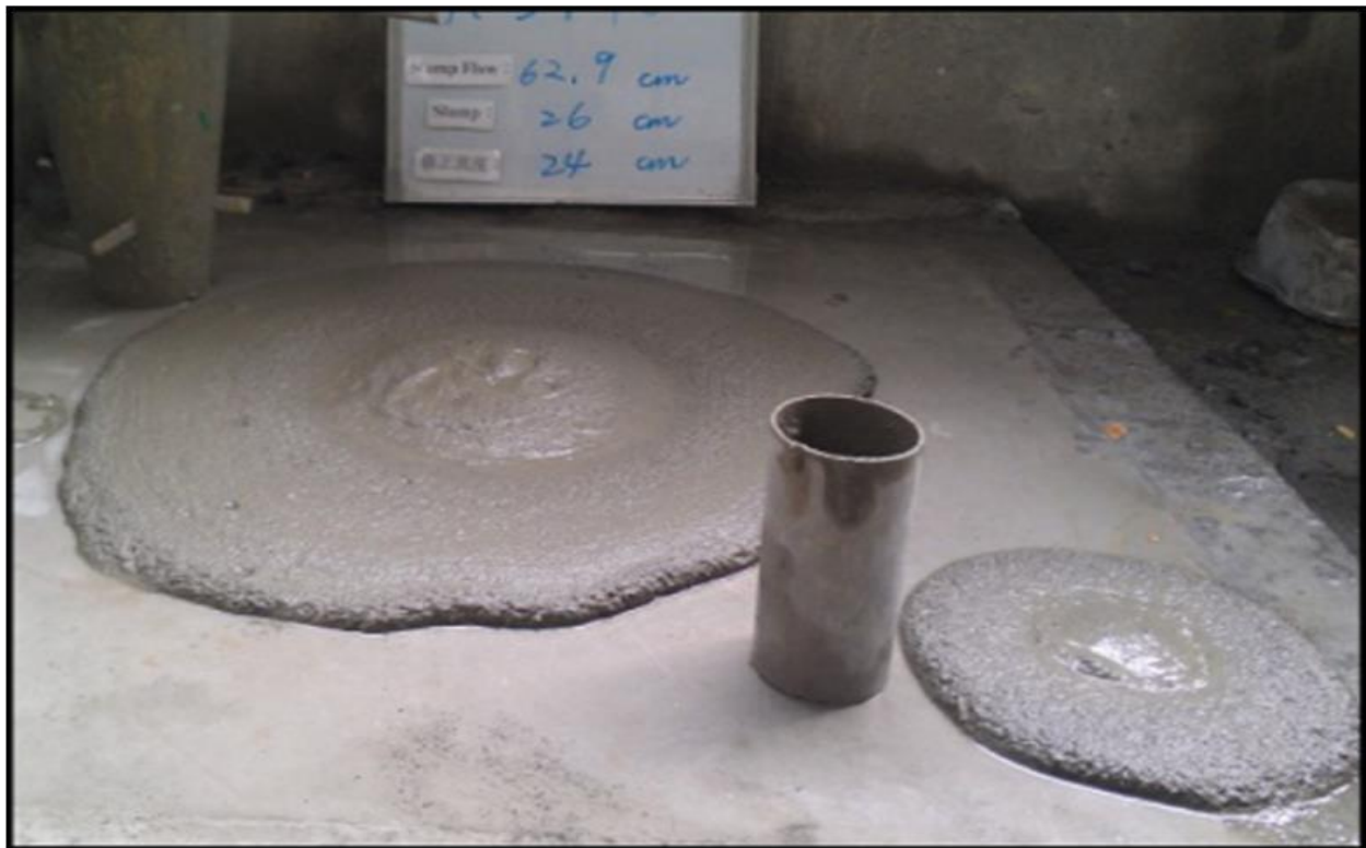
Figure 1.1: Typical spread cone, slump and cylinder slump test (Sheen et al. 2013).
