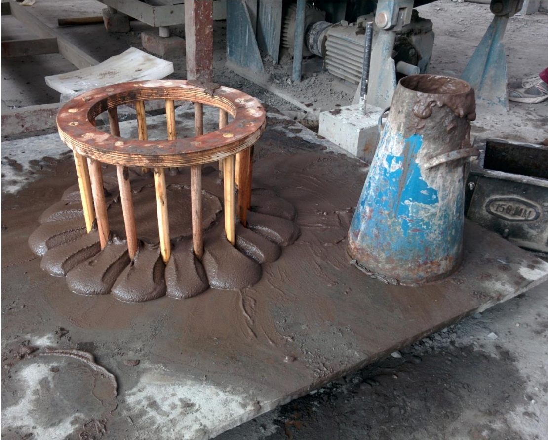
Figure 3.26: J-Ring total flow observed for the mix C/F/G 40A
