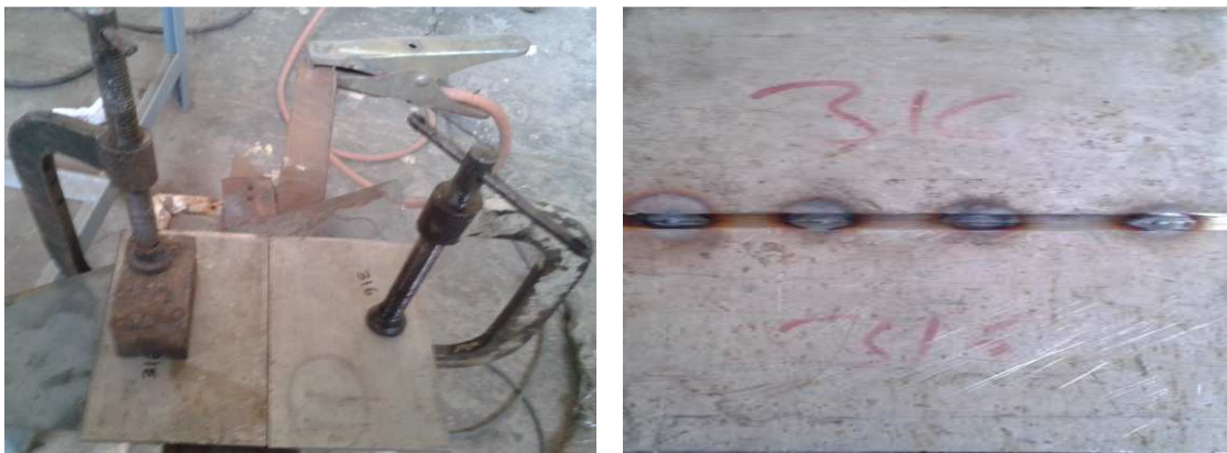
Figure 4.7: Tacking and clamping of samples welded
