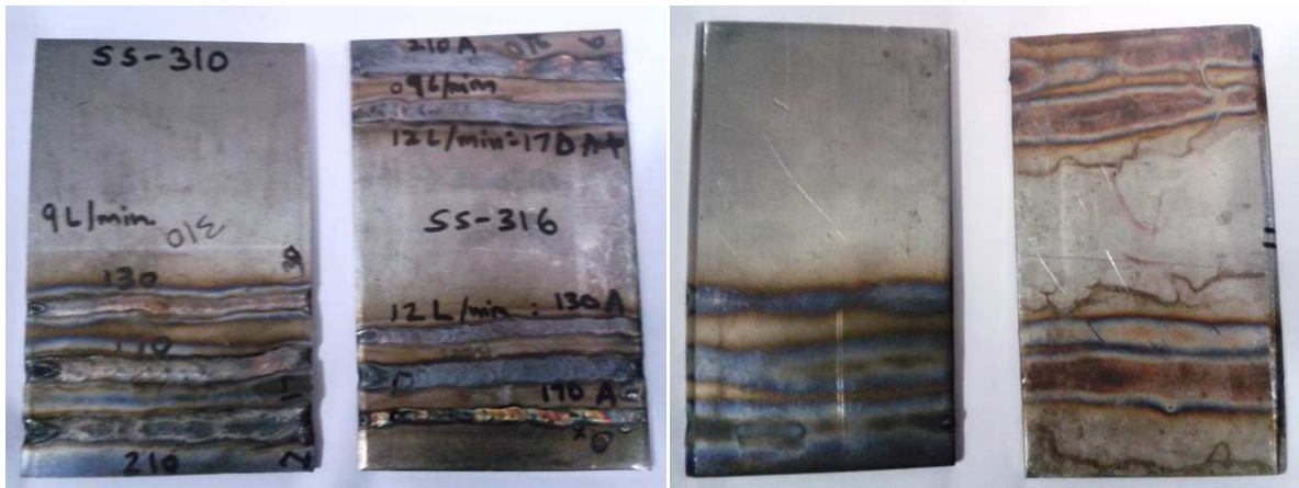
Figure 4.4 Result of pilot study on both SS 310 and SS 316 showing up and down side
