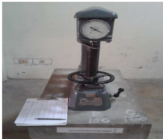
Figure 4.13: Rockwell Hardness Testing machine (Courtesy: solid mechanics lab, Thapar University, Patiala)
