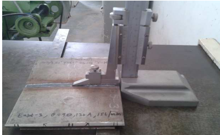
Figure 4.11: Measurement of bead height (Courtesy: workshop at C.E.C, Landran)
