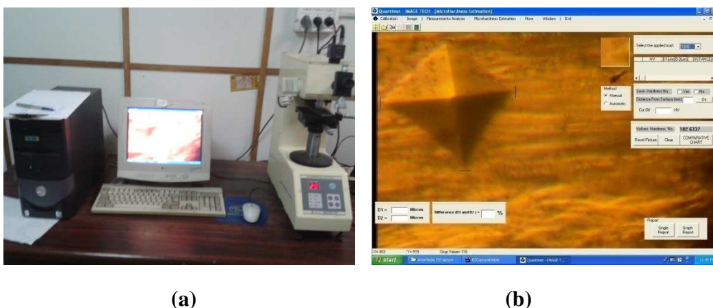
Figure 4.15: (a) Microhardness testing equipment (courtesy Thapar Univ. Patiala) and (b) indentation on one of the sample
