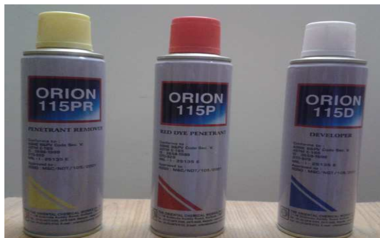
Figure 4.12: Orion’s cleaner, penetrant and developer for DPT of welded specimen.
