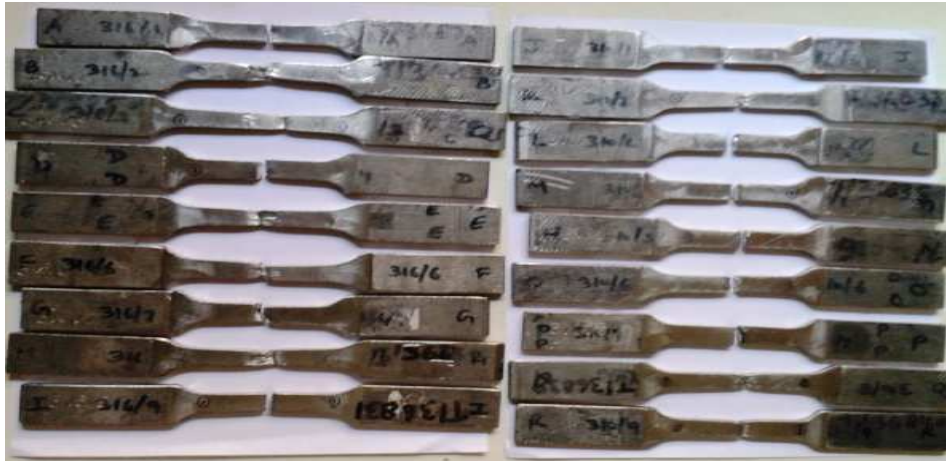
Figure 11.1: Tensile test specimens of both SS 310 and SS 316
