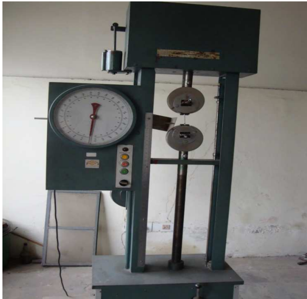
Fig. 6.7 Tensile testing machine used for testing Fig. 6.8 Gripped specimen on the machine
