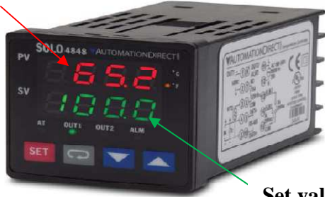
Fig. 4.5 Actual image of the temperature controller showing front and back side
