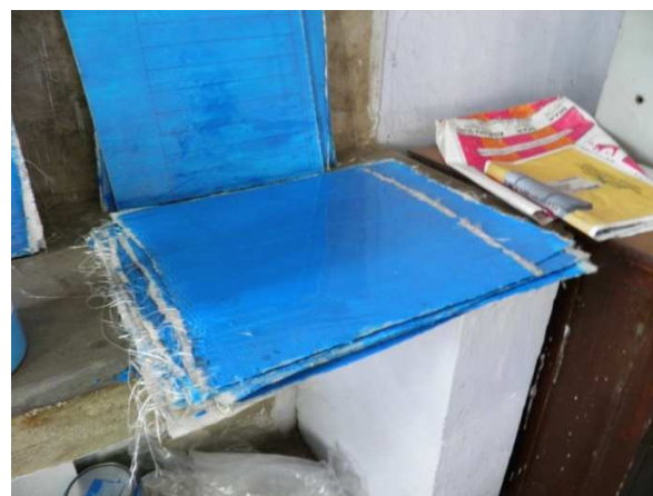
Fig. 4.12 The fully cured sheet with epoxy coating
