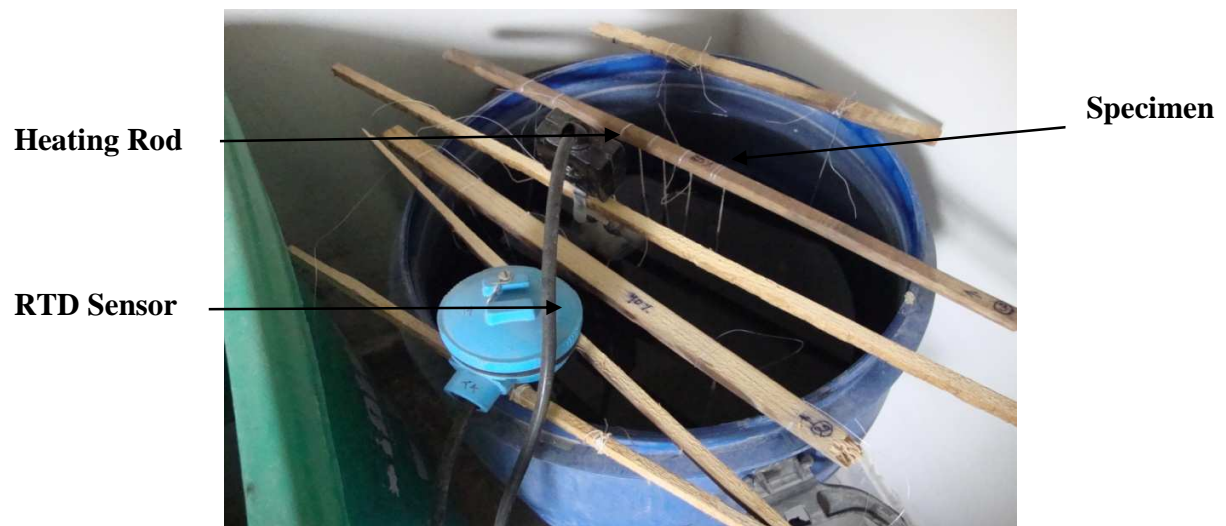
Fig. 4.4 Heating Element and RTD sensor in a tank
