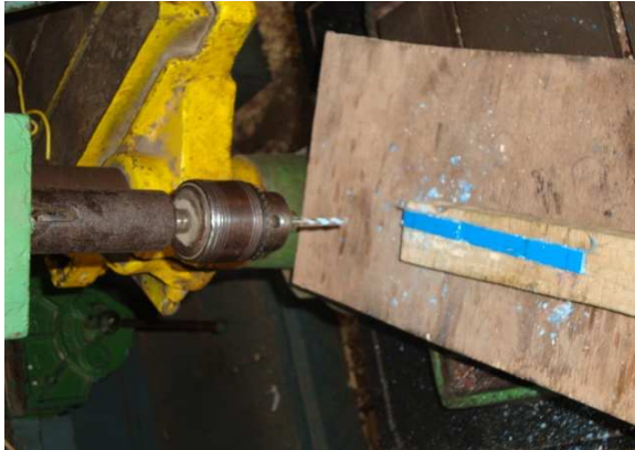
Fig. 4.15 Drilling operation for clamping
