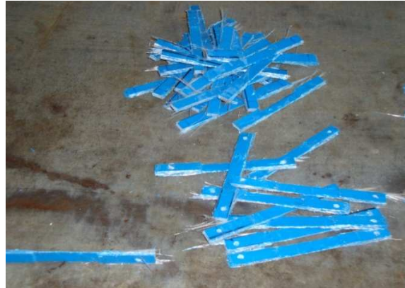
Fig. 4.16 Specimen ready after drilling
