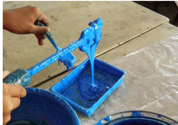
Fig. 4.10 Hand mixing of both base and hardener
