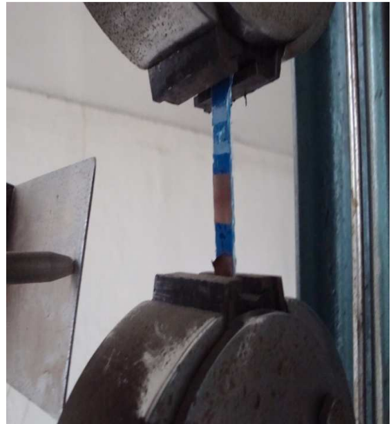
Fig. 6.7 Tensile testing machine used for testing Fig. 6.8 Gripped specimen on the machine
