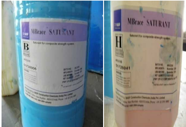
Fig. 4.9 Base (blue colour container) and Hardener (white bottle) used for coating
