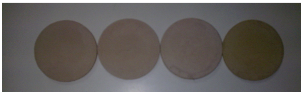
Figure 4.1: Picture of membranes sintered at four different temperature (from left to right 800 °C, 850 °C, 900 °C and 1000 °C)
