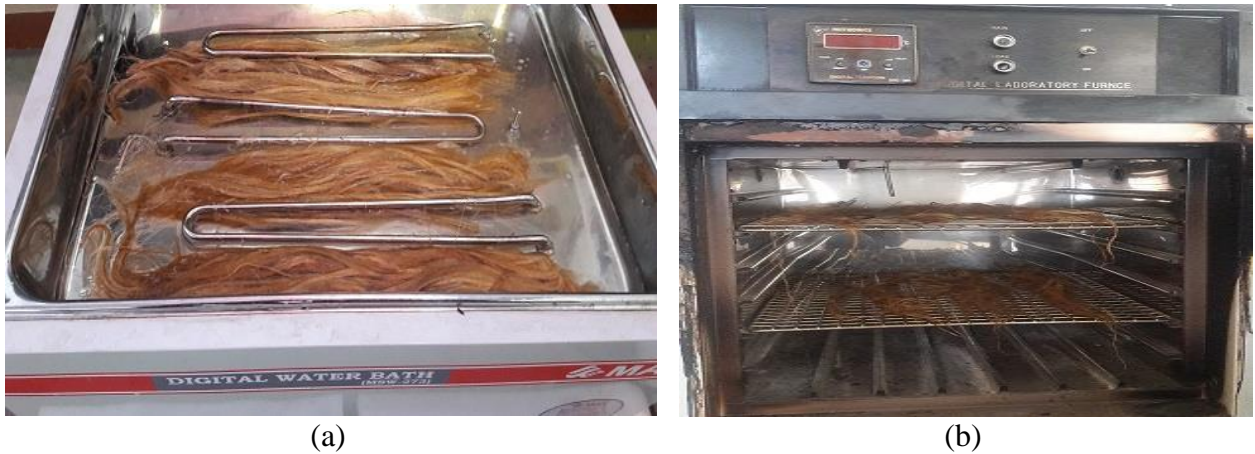
Figure 3.2 Alkali hornification procedure: (a) Wetting process in the water bath at 23°C and (b) Drying process in the furnace at 110°C
