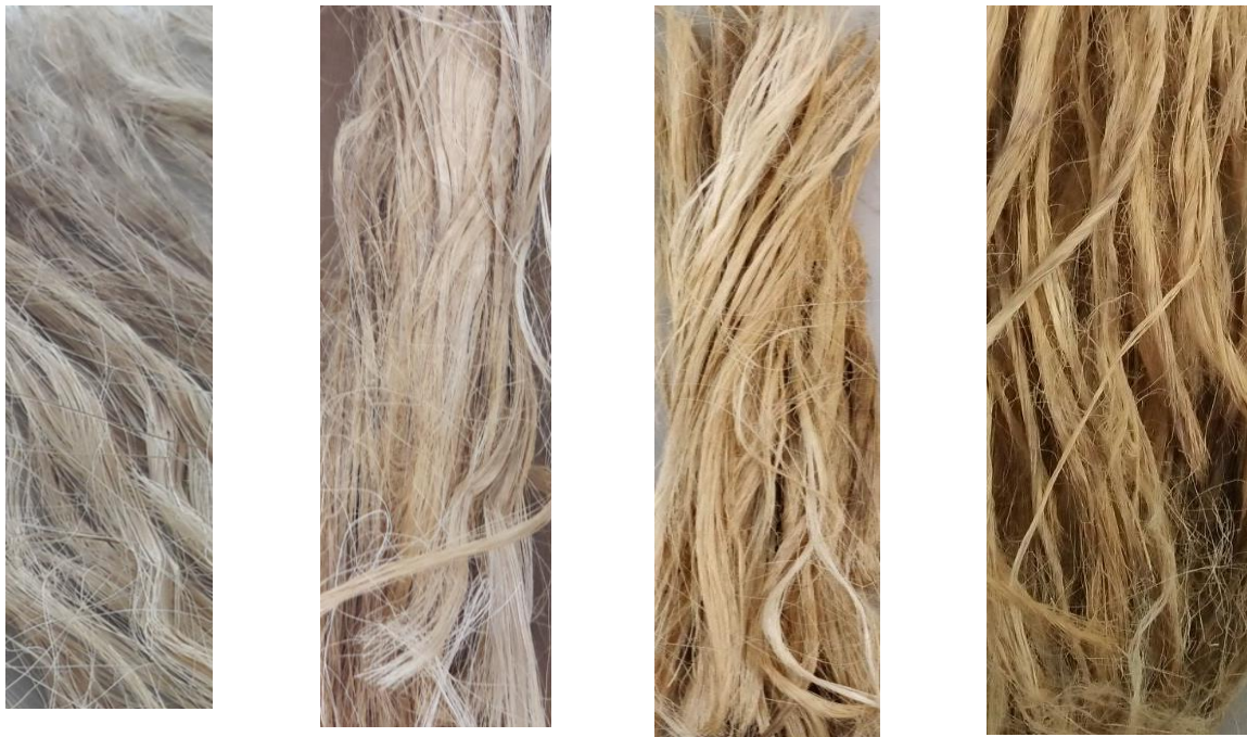
(a) (b) (c) (d) Figure 3.5 Fibre textures after (a) 1 st cycle, (b) 2 nd cycle, (c) 3 rd cycle and (d) 4 th cycle
