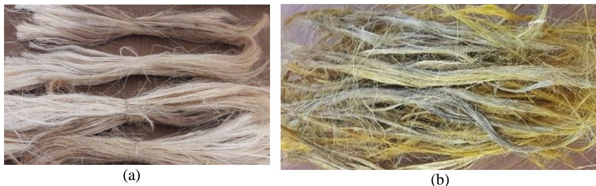
Figure 3.1 Chemical treatments of Agave Americana fibre (a) Untreated fibre and (b) 2% NaOH treated fibre
