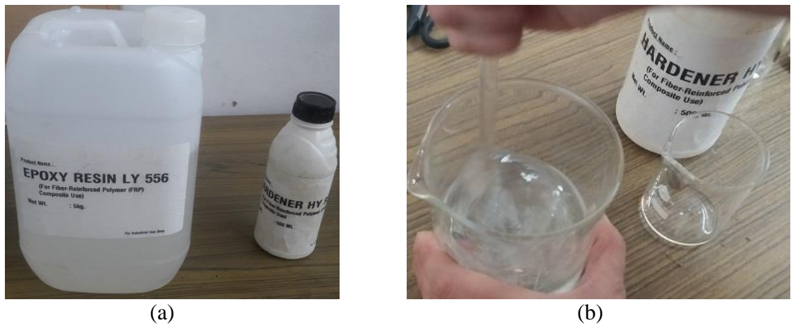
Figure 4.1 Preparation of the resin (a) Epoxy and hardener and (b) Mixing of epoxy and hardener (10:1) with the glass rod
