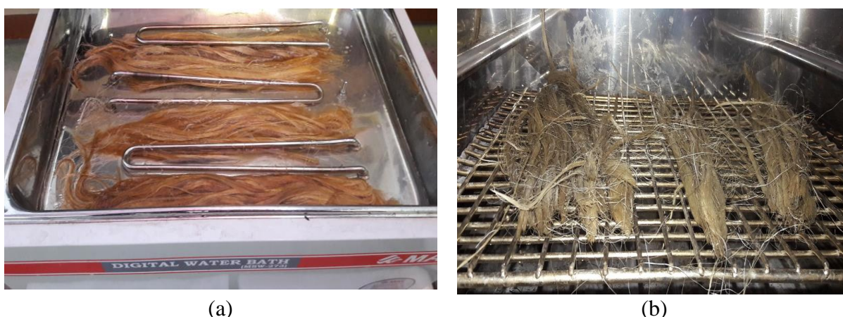
Figure 3.4 Single cycle of water hornification: (a) Wetting process in the water bath at 23°C and (b) Drying process in the furnace (inside view) at 110°C
