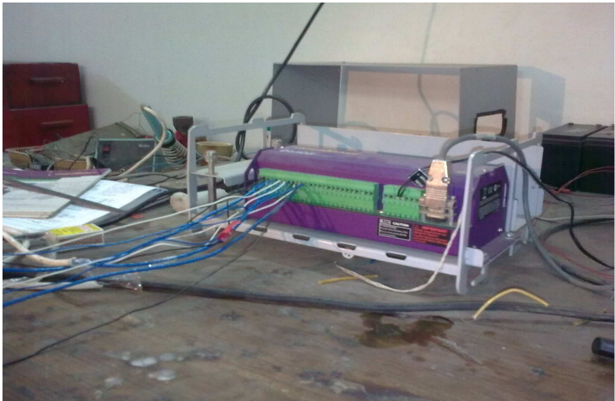
Fig 16. Show the data taker recording the strain
