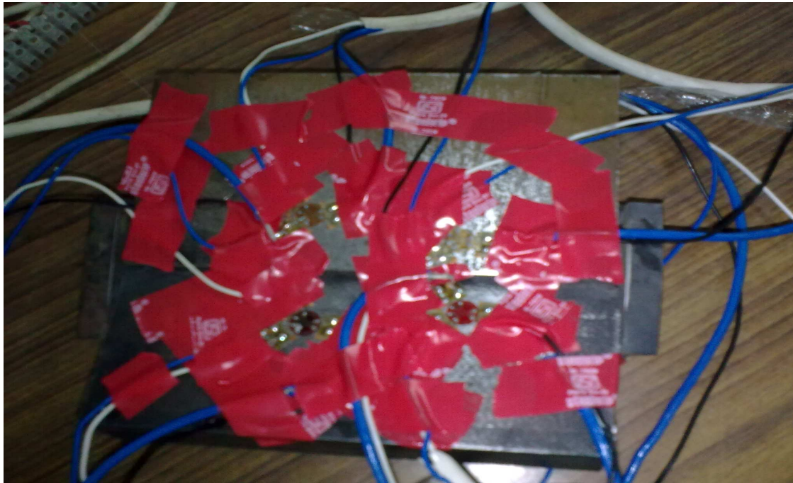
Fig 14: Mounting of strain gauge in weld coupon
