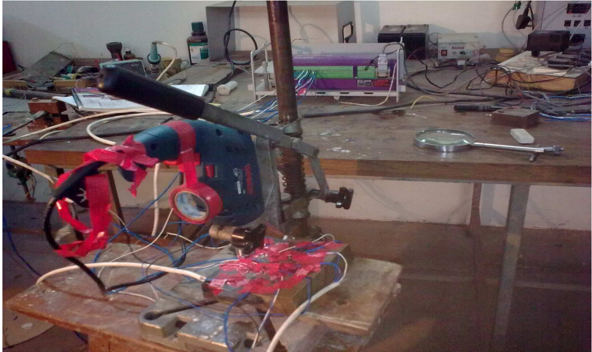
Fig 15: Show the drilling operation during the stress relaxation techniques
