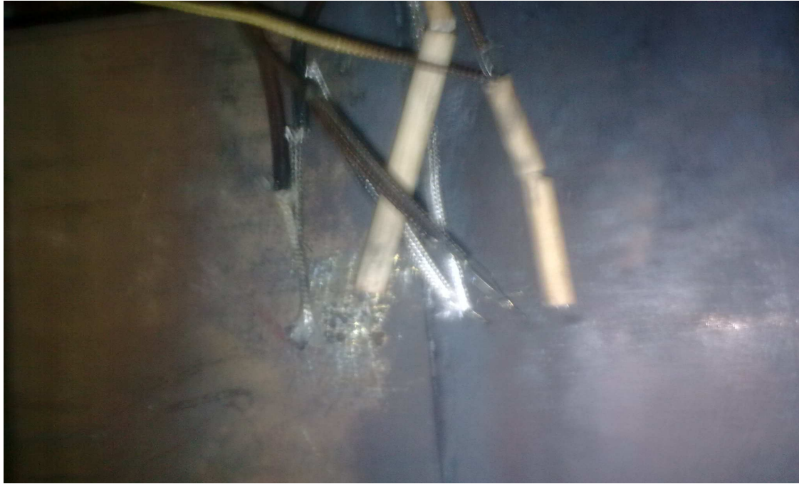
Fig 12 . Mountings of nickel& nickel chromium thermocouples in weld coupon
