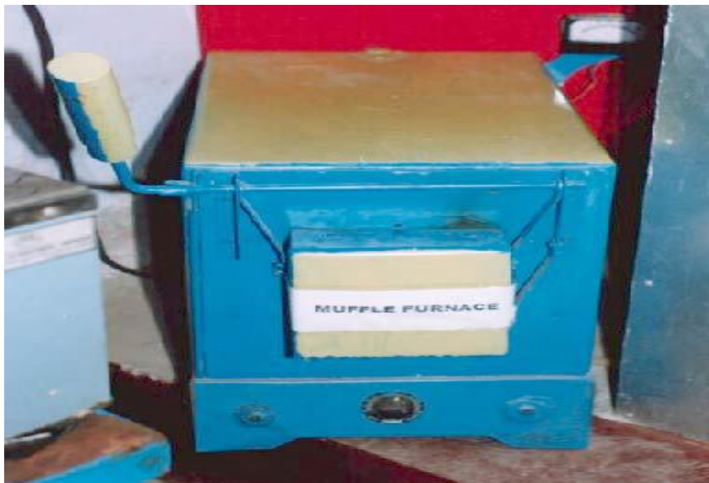
Muffle furnace used for measurement of ash content
