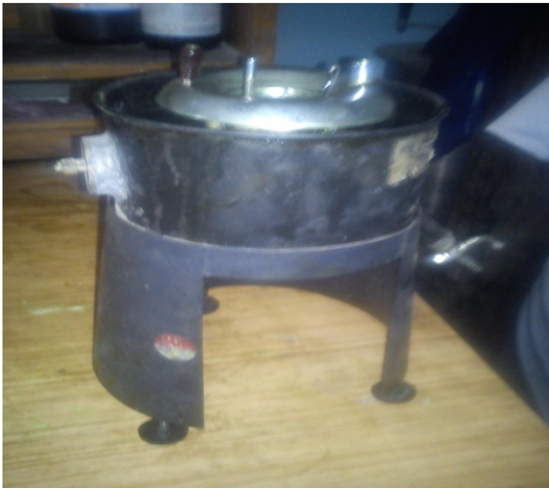
Redwood viscometer used for the measurement of Kinematic viscosity
