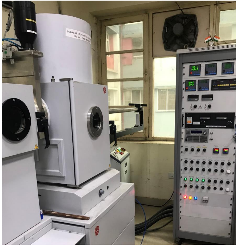
Figure 2.3: RF magnetron sputtering system used for the fabrication of ZnO:Al films.
