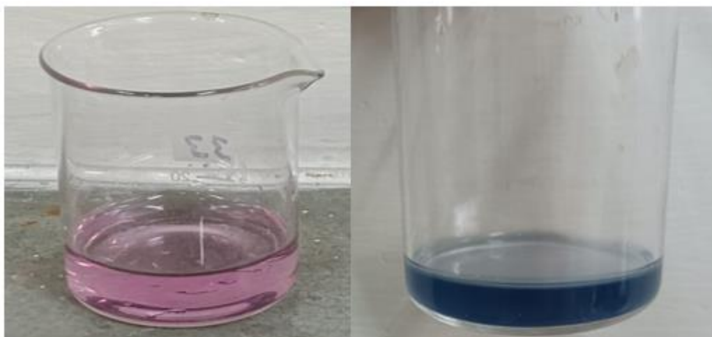
Fig 7. Colour change of indicator from pink to blue during start and end point of titration respectively
