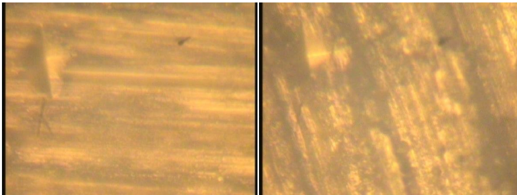
Figure 3.3 Indent mark on steel 304
