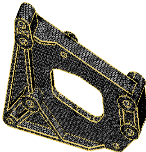
Fig 6.2: Tetrahedral meshing of the modified mounting bracket
