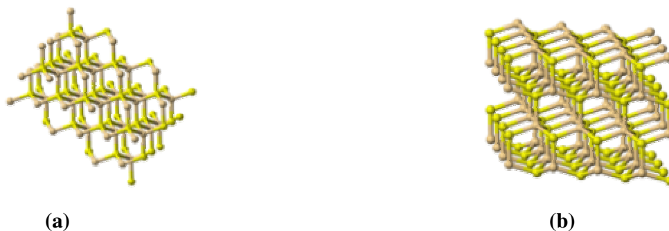
Figure 2.1 (a) 3D model of the structure of hawleyite. (b) 3D model of the structure of greenockite
