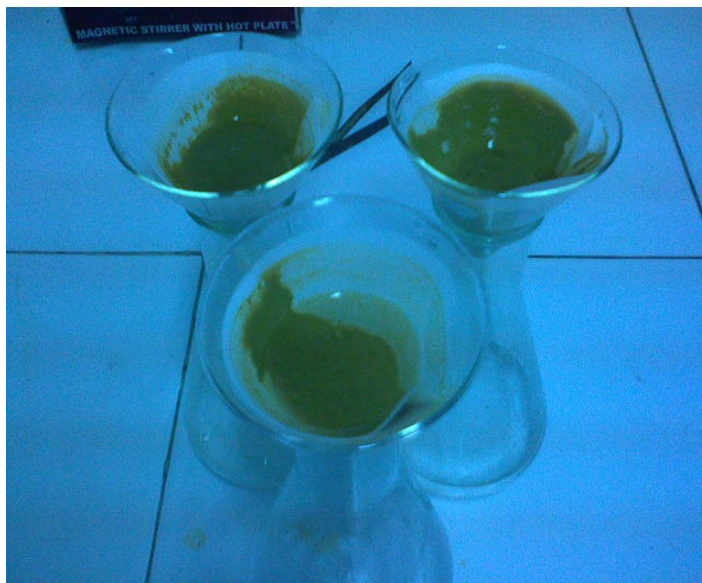
Figure 3.3: Pictorial view of the precipitation process, during the synthesis of Ag doped CdS/Silica nanoparticles
