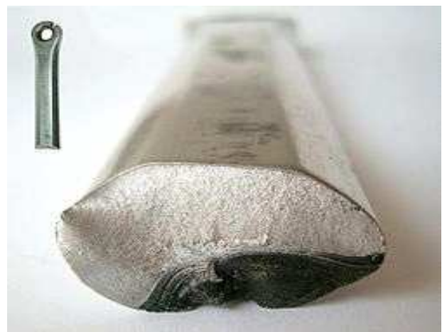
Figure 1.2 Fracture of an Aluminum Crank Arm. Bright: Brittle fracture, Dark: Fatigue fracture.
