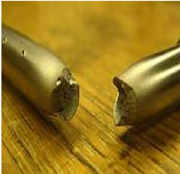
Figure 1.3 Ductile Failure of a Specimen Strained Axially.
