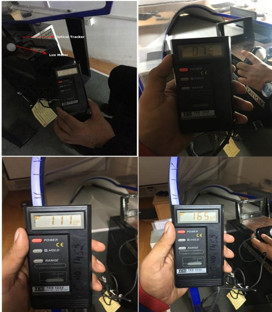
Figure 5.31: Readings of Lux meter under different light intensities
