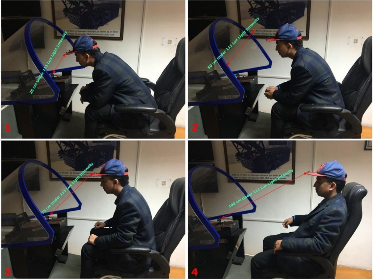
Figure 5.34: Experiment conducted at light intensity value of 111 lux light intensity at different distances: 25 cm, 50 cm, 75 cm & 100 cm marked 1-4 respectively
