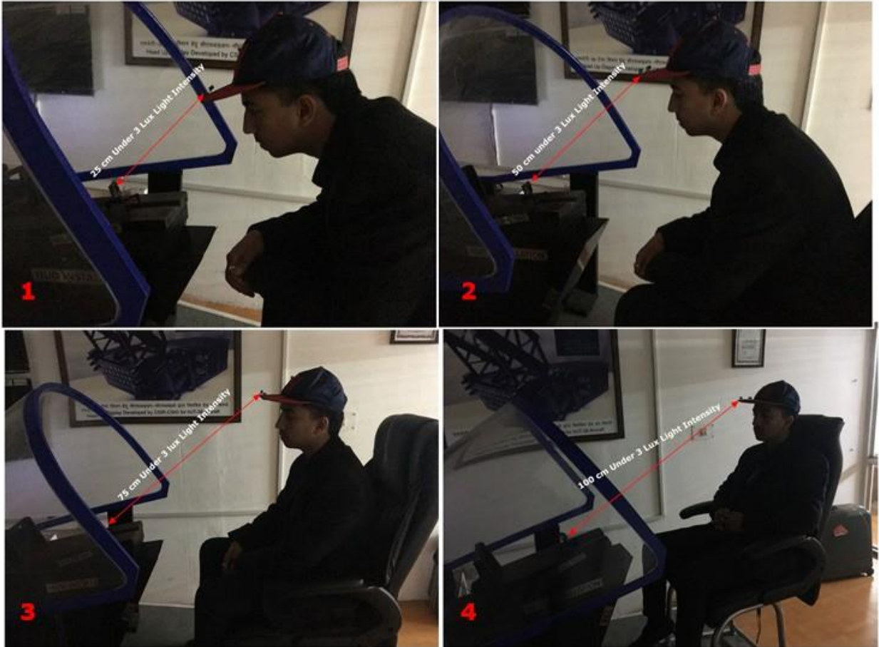
Figure 5.32: Experiment conducted at light intensity value of 3 lux at different distances: 25 cm, 50 cm, 75 cm & 100 cm marked 1-4 respectively
