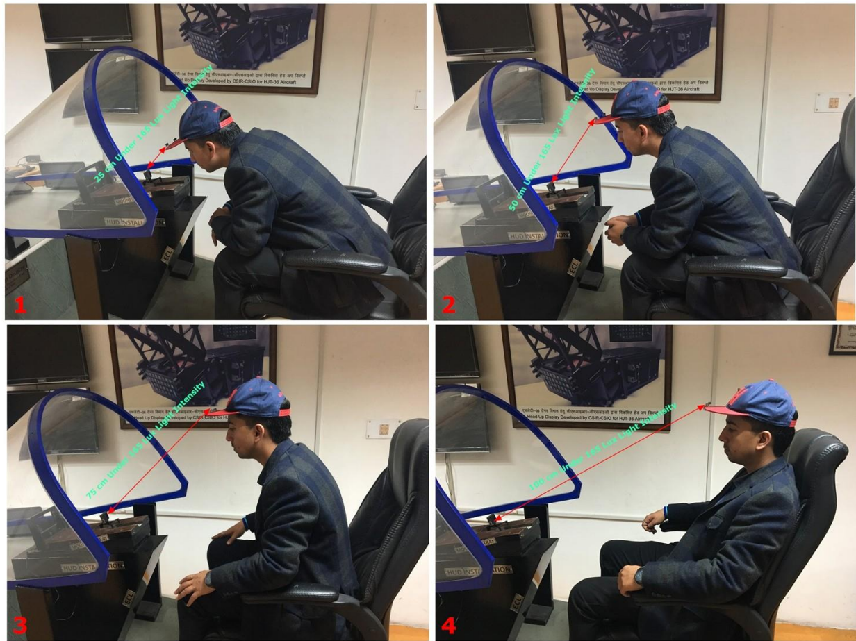
Figure 5.35: Experiment conducted at light intensity value of 165 lux light intensity at different distances: 25 cm, 50 cm, 75 cm & 100 cm marked 1-4 respectively
