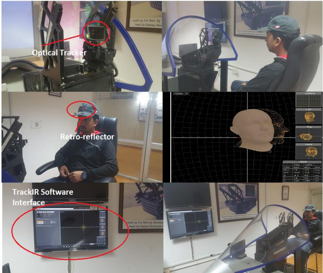
Figure 5.36: Experimental setup of the optical tracking system with the software interface
