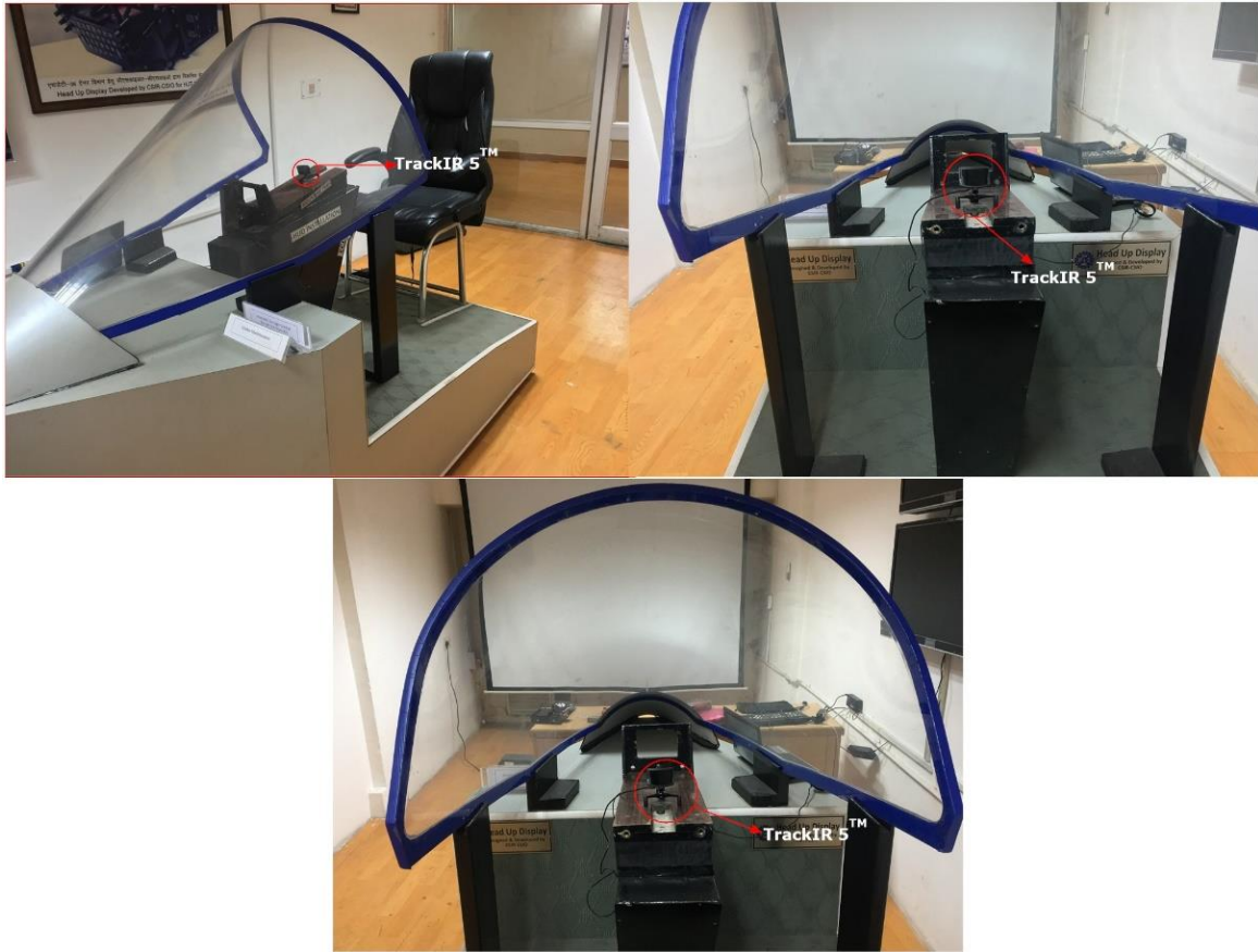
Figure 5.30: Cockpit Simulator with Optical Tracker TrackIR 5 TM (encircled in red) at CSIR-CSIO, Chandigarh, India
