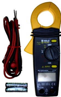
Figure5.3 Clamp-on current transducer
