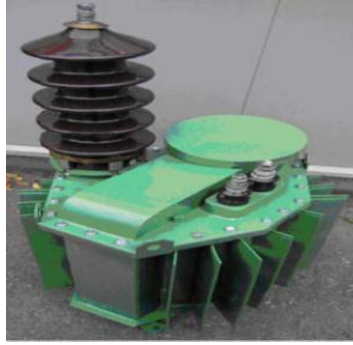
Figure 1.11 Phased transformers with ferrofluid coolant system
