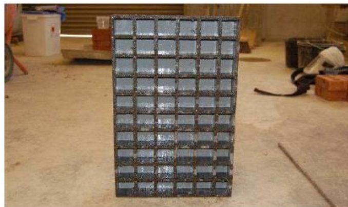
Fig. 3.17 Fabrication of the grating specimen (Gai et al., 2009)
