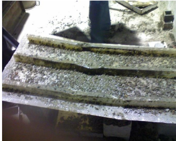
Fig 3.20 Buckling of channels (Reema, 2010)
