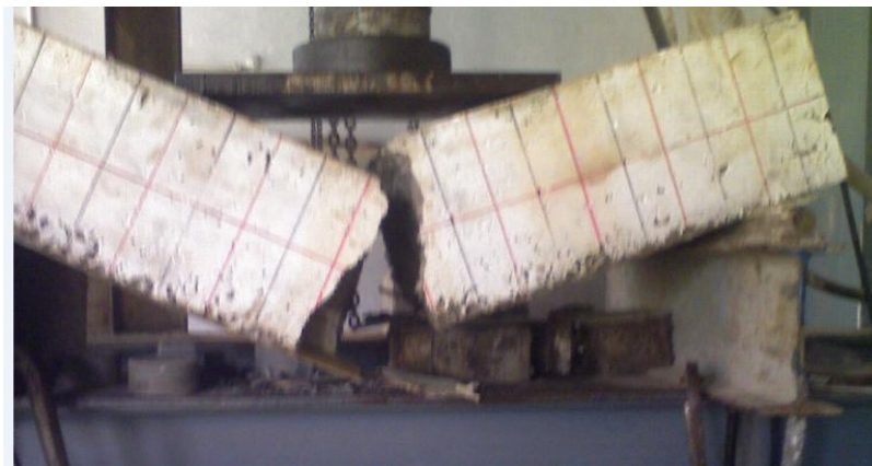
Fig 3.21 Sudden brittle failure (Reema, 2010)
