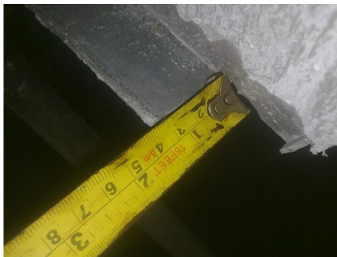
Fig 6.3 debonding in specimen 1
