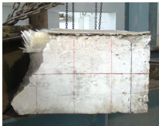
Fig 3.22 Debonding of form (Reema, 2010)
