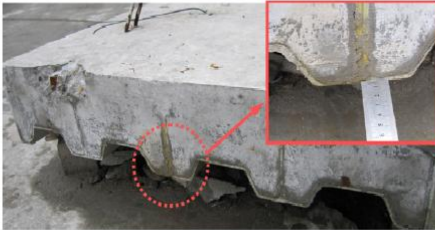
Fig 3.24 Relative slip at the end of specimens, bonded (He et al., 2012)
