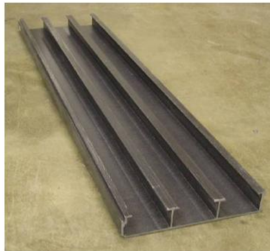
Fig. 3.4 12 inches wide pultruded FRP plank (Bank et al., 2007)
