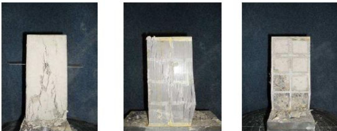
Fig. 3.27 Failure of block specimens (Gai et al., 2011)
