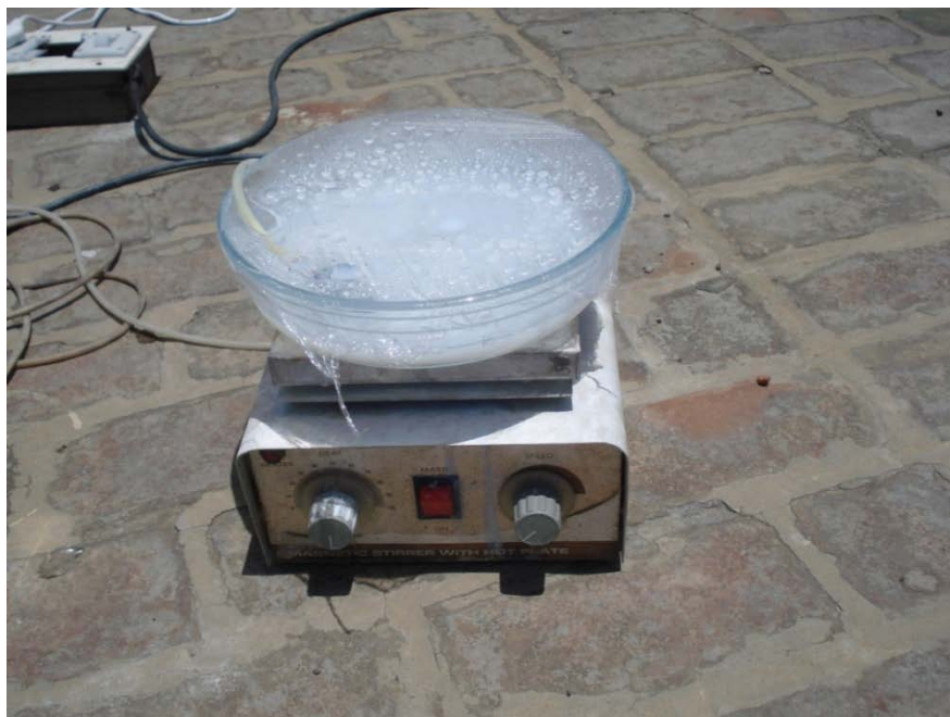
Figure -4.8 Glass bowl reactor magnetic stirrer under sun light
