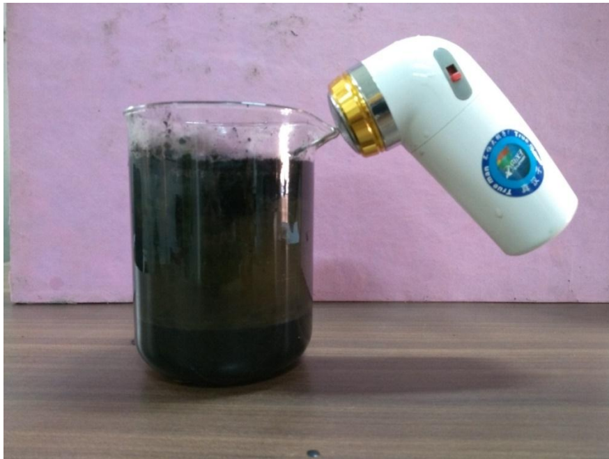
Figure 4.3: Uniform mixing of coal sample with stirrer
