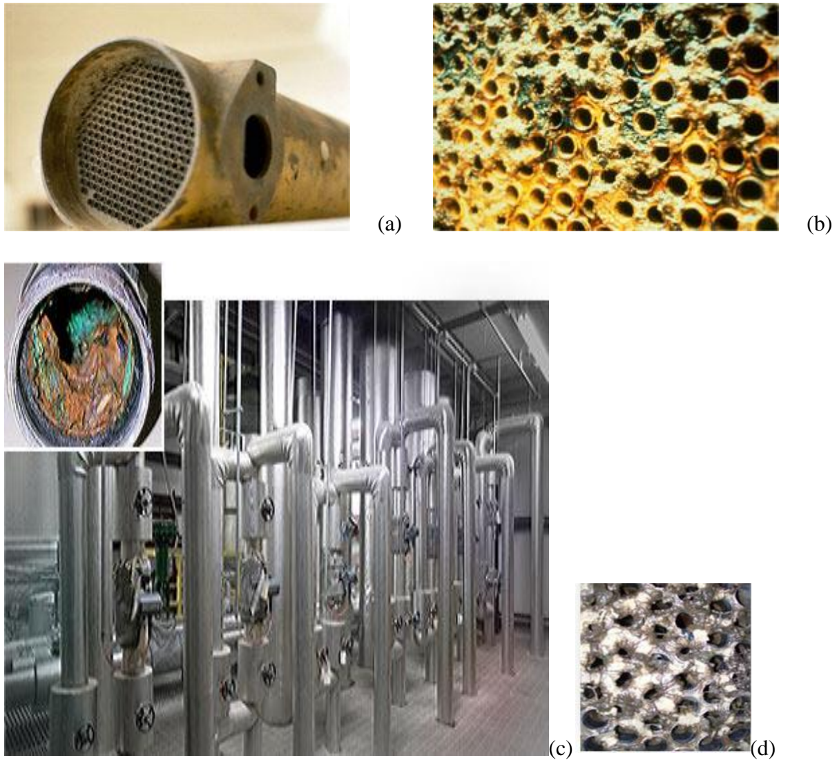
Figure 2.6 Impact of biofilm formation in Industrial units. The figure shows (a) Heat plant circulation systems; (d) Biofilm affected cooling tower of a waste water treatment plant (Lequette et al , 2010)exchanger of the type used in the emergency cooling water systems of nuclear power plants (b) The same type of heat exchanger heavily fouled with biofilm deposits. Such deposits can severely reduce the heat transfer capacity of heat exchangers thereby impacting the safe operation of emergency cooling water systems in power plants; (c) Biofilm in stainless steel pipe. This type of large-scale biofouling is common in many industrial water system components including, pulp and paper manufacturing, cooling towers, and nuclear power
