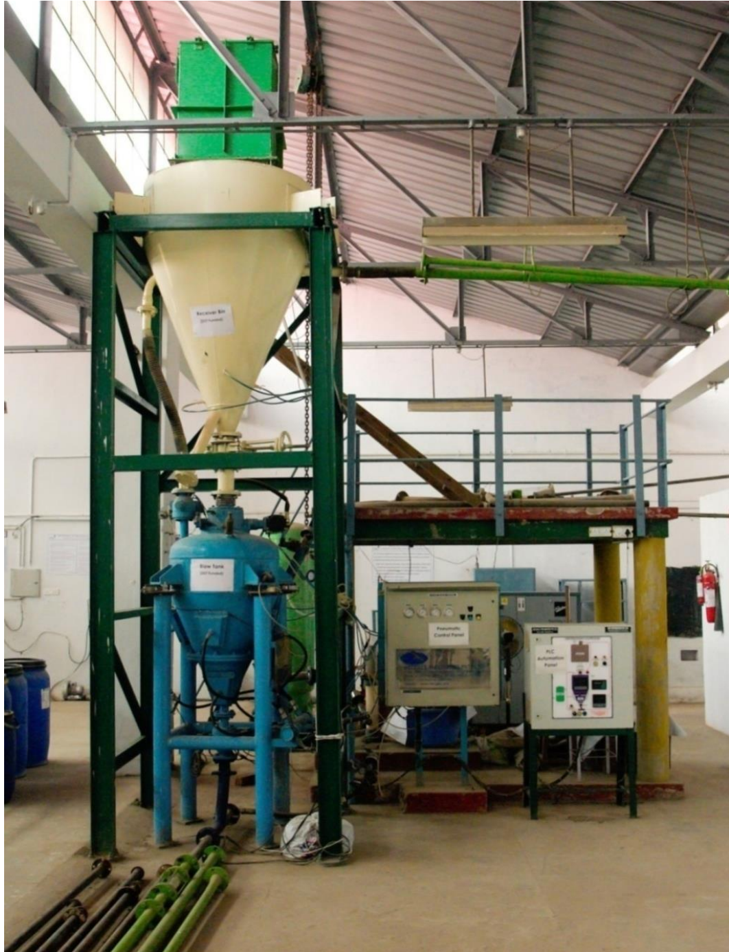
Figure 3.1: A view of the blow tank together with the receiving tank
