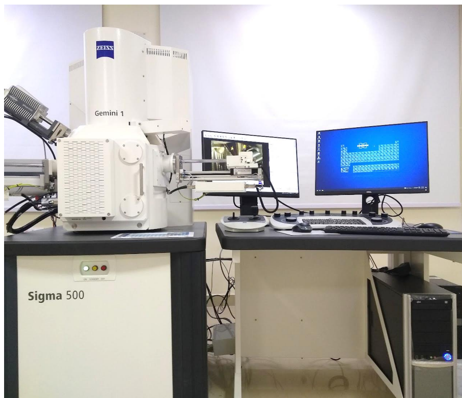
Figure A-2 Scanning Electron Microscopy (Make: Sigma - ZEISS Field Emission SEM, Photo Courtesy: Electron Microscopy laboratory, TIET, Patiala)
