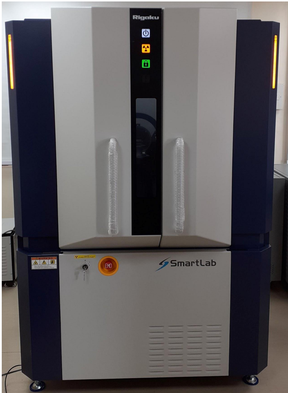
Figure A-3 X-Ray Diffractometer (XRD) (Make: SmartLab Rigaku, Japan, Model: SmartLab SE, Photo Courtesy: School of Physics and Materials Science, Thapar Institute of Engineering & Technology)
