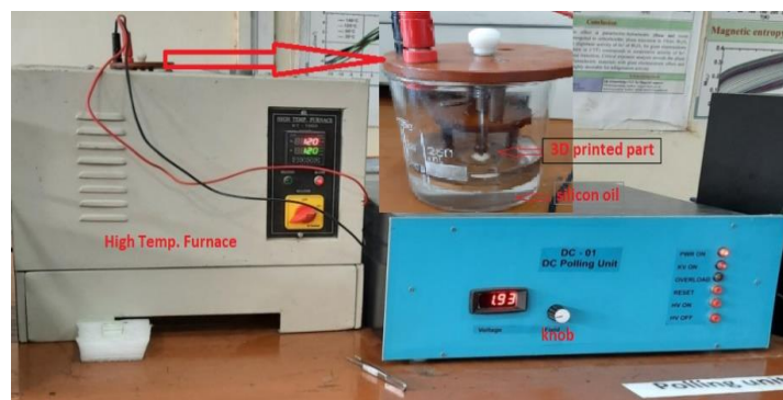
Figure 3.11 Setup used for electrical poling of specimen
