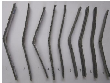
Figure 5.17 Fractured samples after destructive testing
