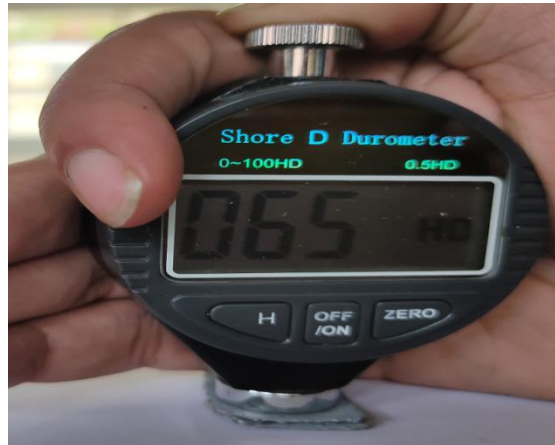
Figure 4.14 Shore D Durometer used for hardness testing
