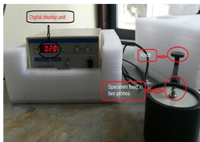
Figure 5.62 D_{33} meter used to measure piezoelectric coefficient
