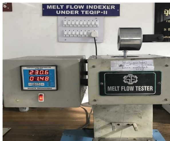
Figure 4.1 Melt flow tester used for flowability check
