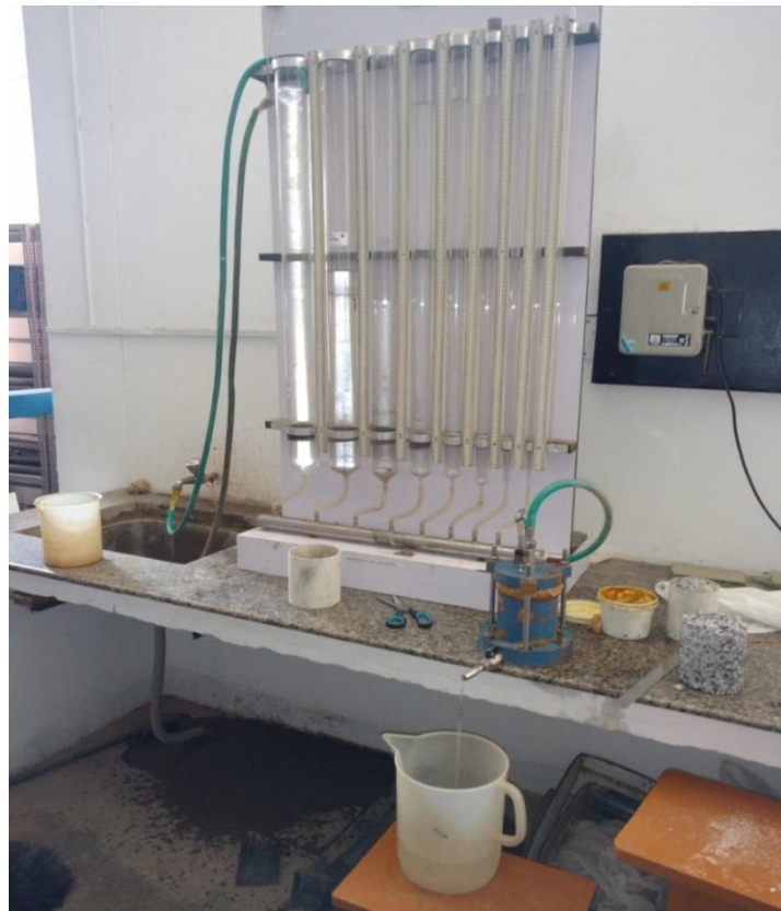
Figure 3.10 Permeability test setup.
