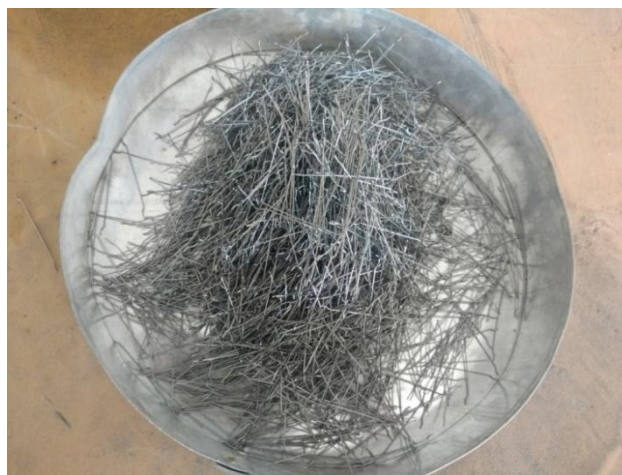
Figure 3.4 Steel fibres used in this study
