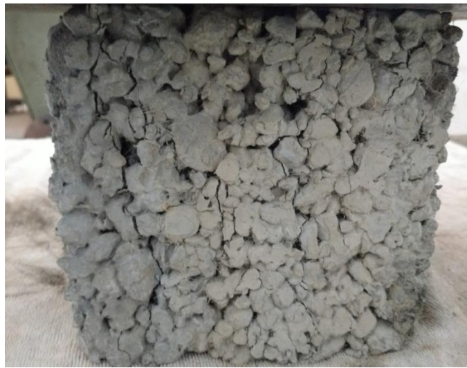
Figure 4.2 Failed Sample in Compressive strength test.
