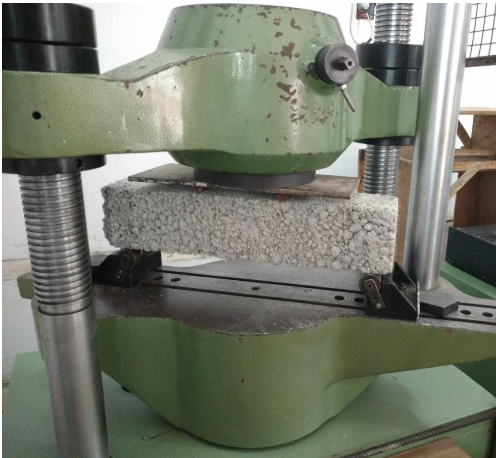
Figure 3.7 Flexural Strength test setup.
