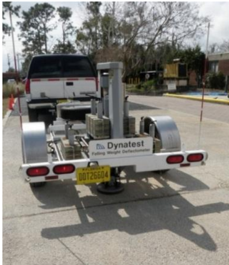
Figure 2.2: Falling Weight Deflectometer (FWD) [9].
