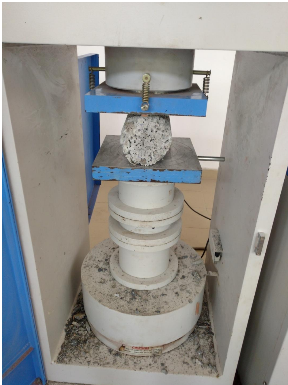
Figure 3.8 Split Tensile Strength test setup.
