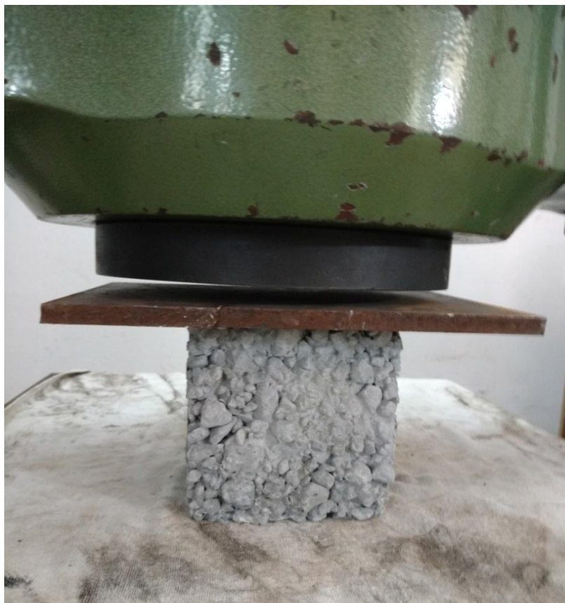
Figure 3.6 Compressive Strength testing setup.
