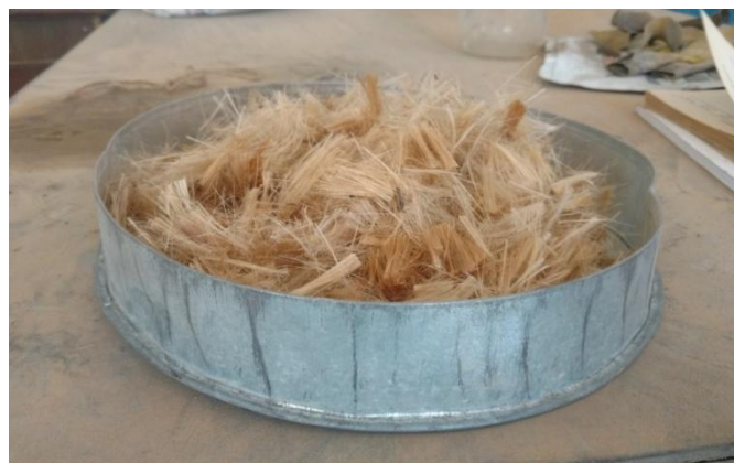
Figure 3.3 Jute Fibres used in this study.
