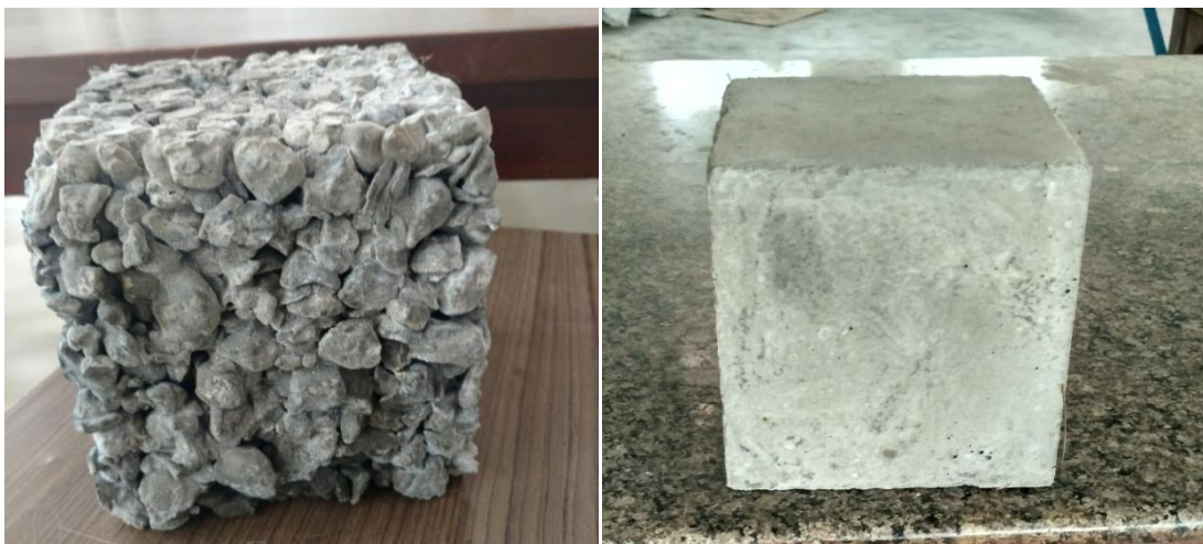
Figure 1.1 (a) No-Fines Concrete.
