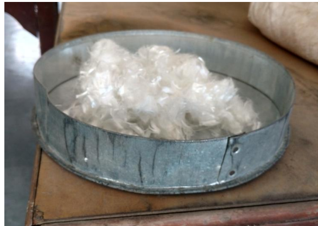
Figure 3.2 Polypropylene Fibres used in this study.
