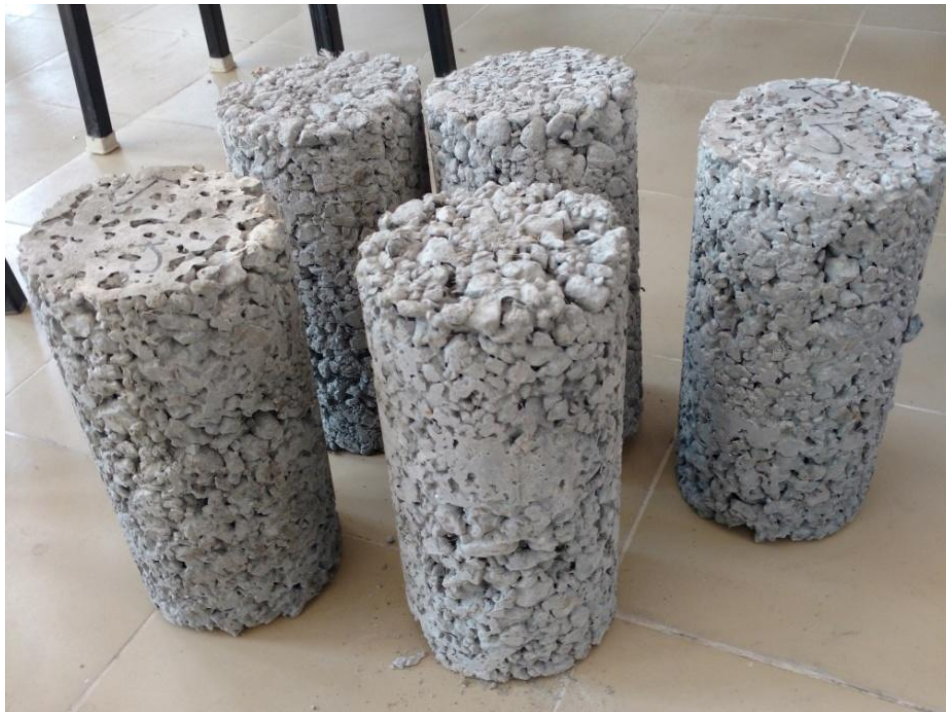
Figure 3.5 Demoulded Concrete Samples.
