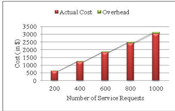
Figure 3.7: Overhead of Layered Architecture
