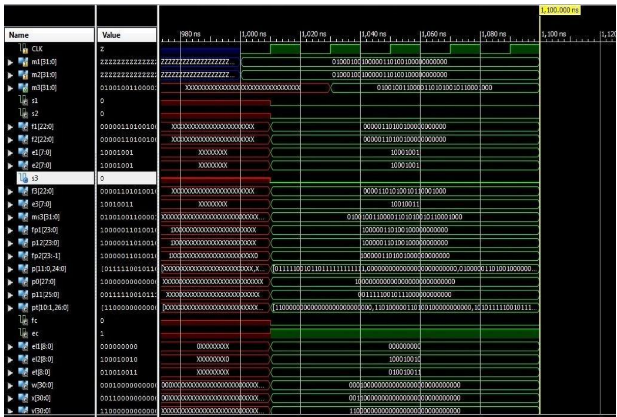
Figure 5.3 Simulation result for floating point multiplier
