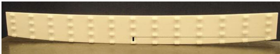
Figure 1.8: Curling of part at corners [13]
