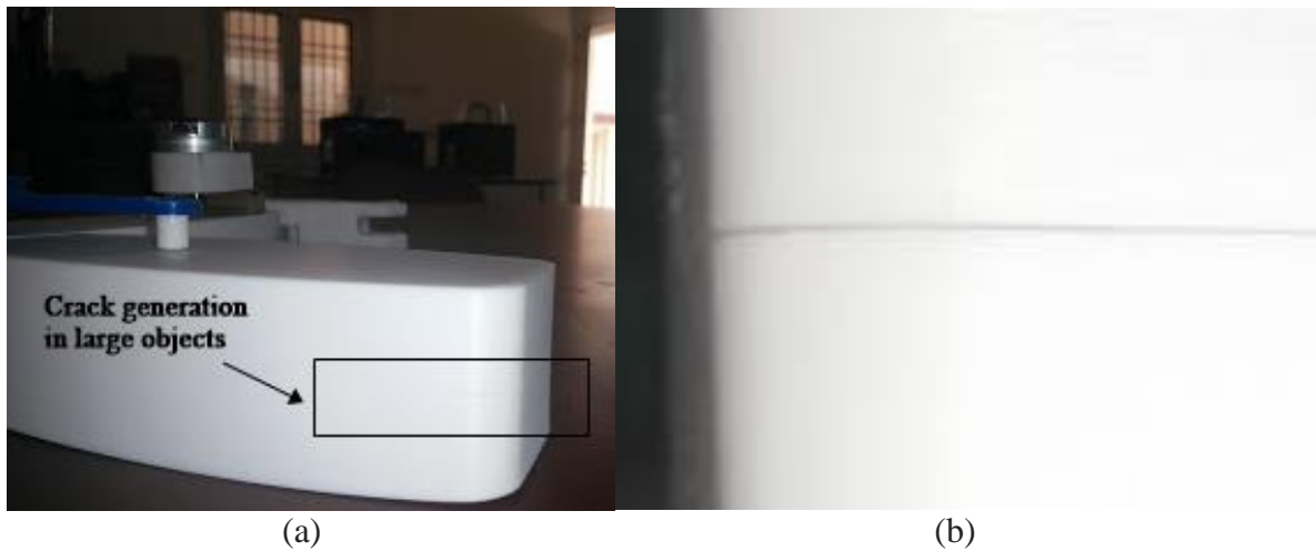
Figure 5.9: (a), (b) Cracks in tall objects
