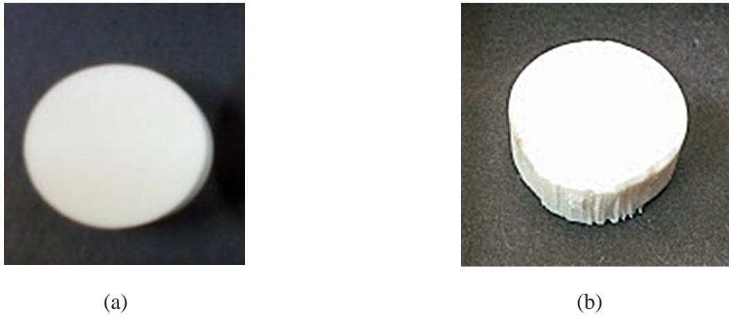
Figure 5.5: (a) Part oriented to vertical central axis, (b) Part oriented to horizontal central axis
