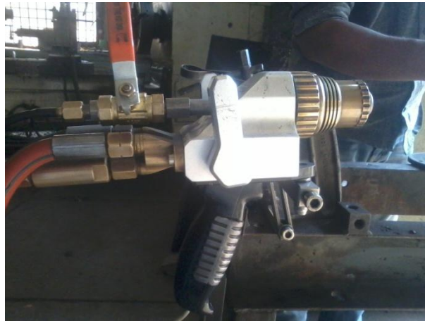
Fig. 3.8: Gun used for HVOF coating
