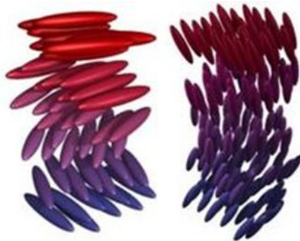
Fig. 3.4 The chiral nematic phase (left), also called the cholesteric phase, and the smectic C* phase (right)
