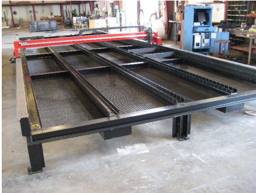
Fig.1 Plasma arc cutting table with moving torch.
