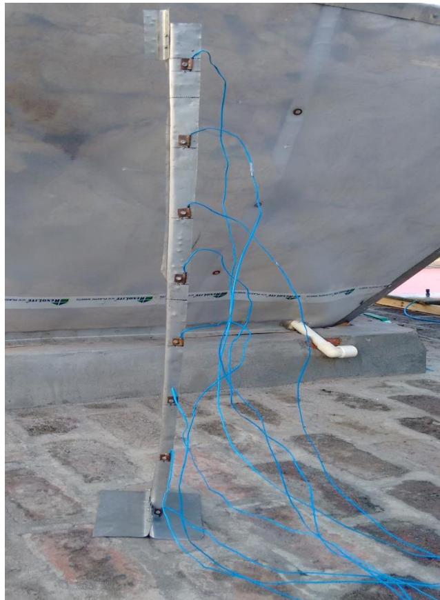
Figure 3.3 Eight T-type thermocouples with stainless steel frame
