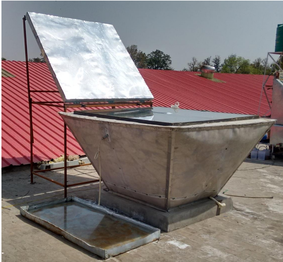
Figure 3.1 shows the snapshot of trapezoidal salt gradient solar pond (TSGSP)
